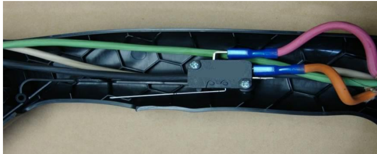
Fig. 6-15 Switch Wire Location
