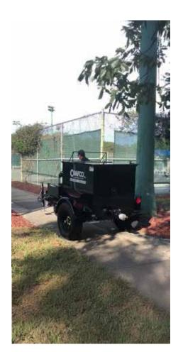
The EZ Paint Mixer combines power, mobility and safety to make any paint or industrial coating project easier. A high-torque hydraulic drive powers through viscous fluids and added fillers. Get precise mixing control for proper material performance with the EZ Paint Mixer's variable speed agitator and full-sweep mixing paddles.
