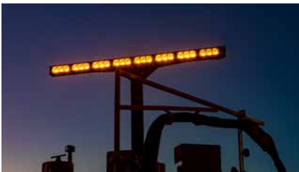
Arrow Bars (Unclassified) Wide flashing multiple LED bar with programmable directional flash patterns and two brightness levels w/ included control box.
