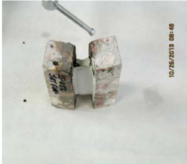
Figure 4 - RoadSaver Silicone Non-Sag Test Specimen - After Fluid Test
