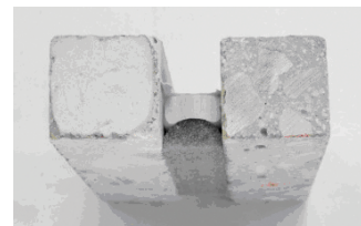
Figure 3 - RoadSaver Silicone Non-Sag Test Specimen - During Fluid Test
