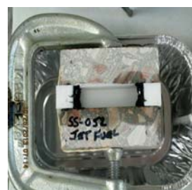
Figure 3 - RoadSaver Silicone Non-Sag Test Specimen - During Fluid Test
