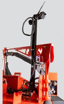
**Telescoping mast and adjustable camera** expands the field of vision.
