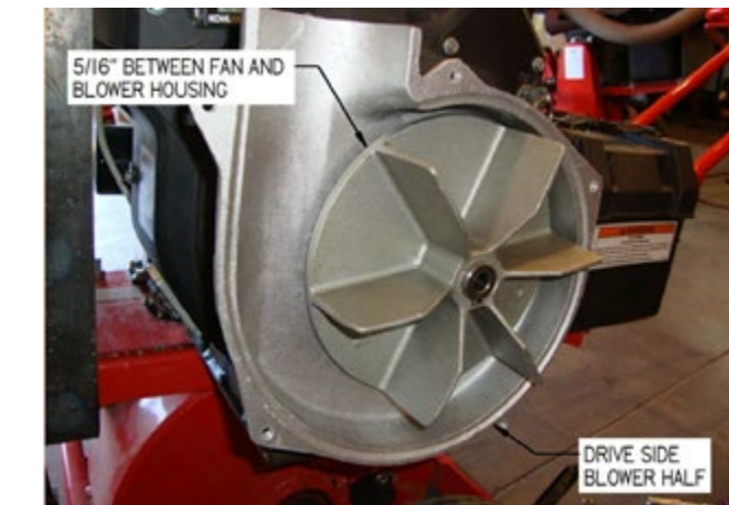
Figure 6-16 Blower Fan Installation
