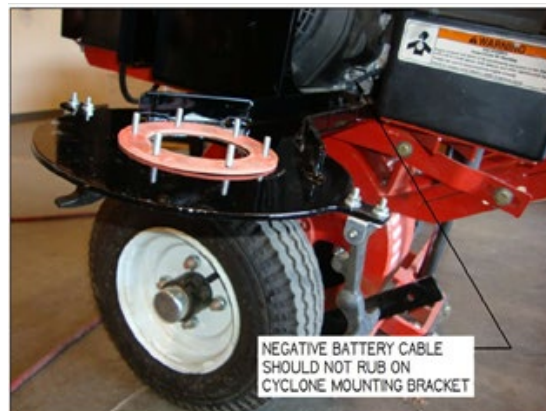
Figure 6-14 Cyclone Mounting Plate Installation
