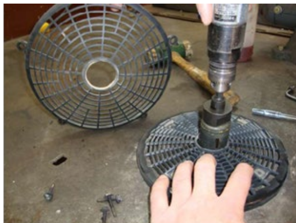
Figure 6-2 Flywheel Cover and Grass Screen Hole Cutting
