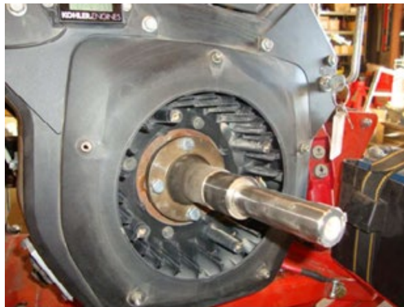
Figure 6-1 Kohler Front Drive Shaft Installed
