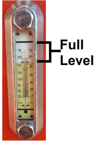
Figure 5-2 Hydraulic Fluid Level and Temp Gauge
