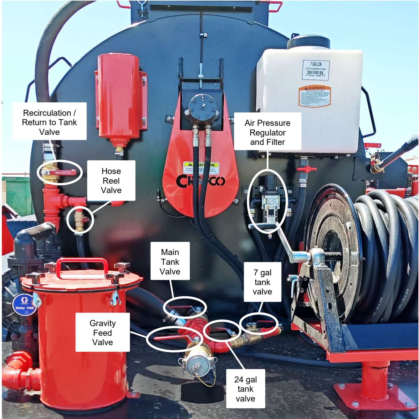
Figure 5-1 Sealcoater Valves and Water Hose (See detail view next page.)
