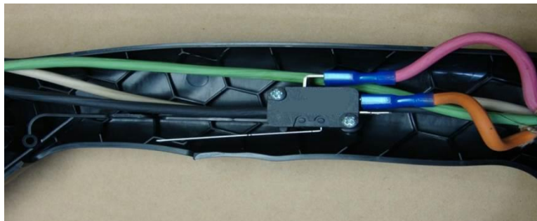
Fig. 6-4 Switch Wire Location
