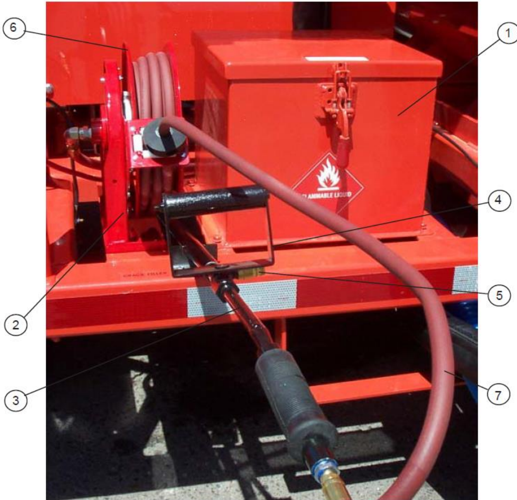
Figure 9.25 Crack Sealing Attachment
