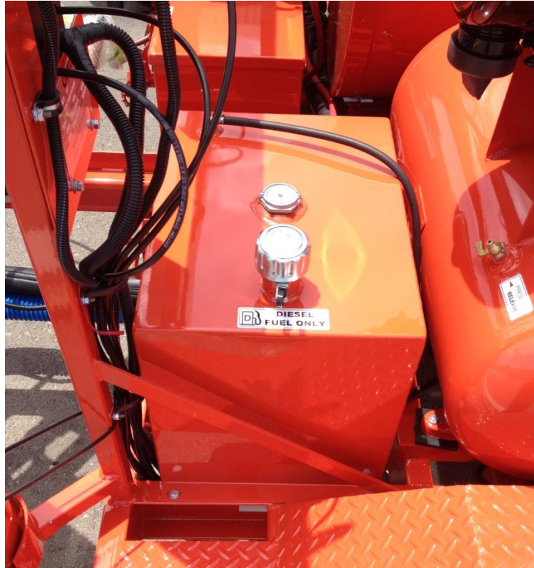
Figure 5.1 Diesel Fuel Fill Cap and Level Gauge
