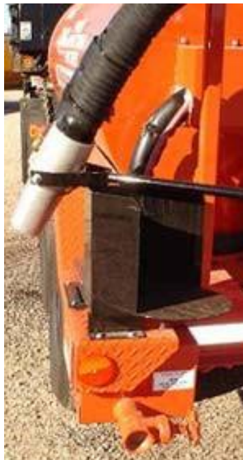
Figure 5.6 Nozzle Removed from Flush Box
