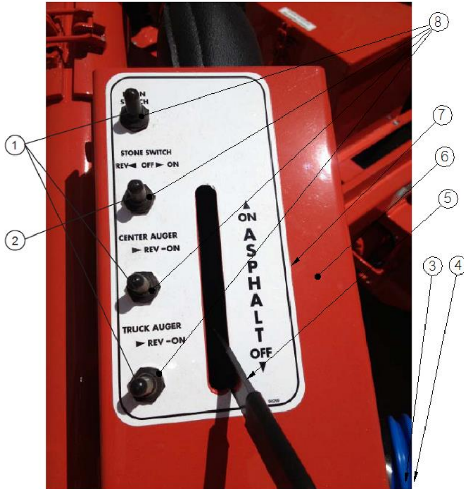
Figure 9.18 Boom Control Console
