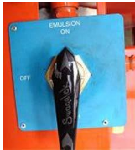
Figure 5.9 Emulsion Tank Valve
