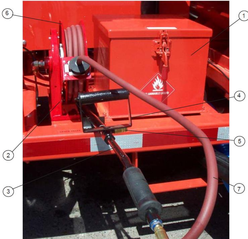
Figure 9.25 Crack Sealing Attachment
