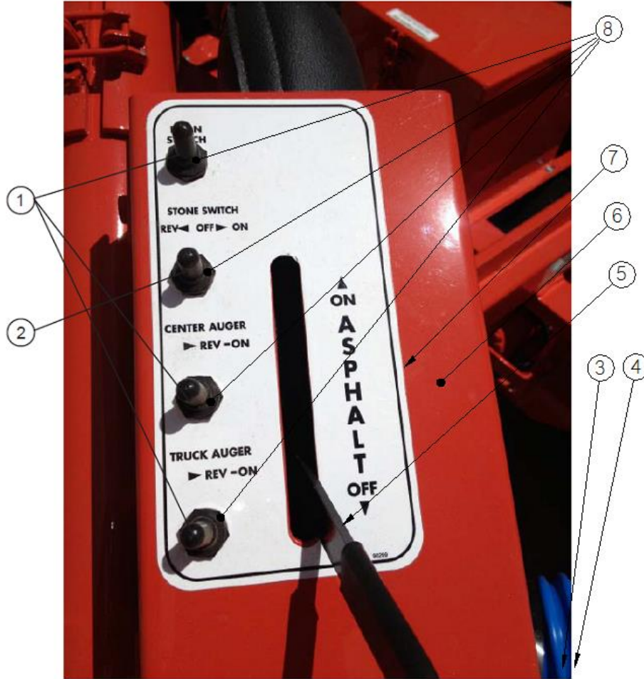
Figure 9.18 Boom Control Console
