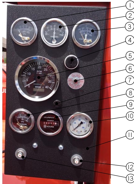
Figure 9.22 Engine Control Panel
