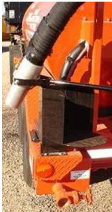
Figure 5.6 Nozzle Removed from Flush Box
