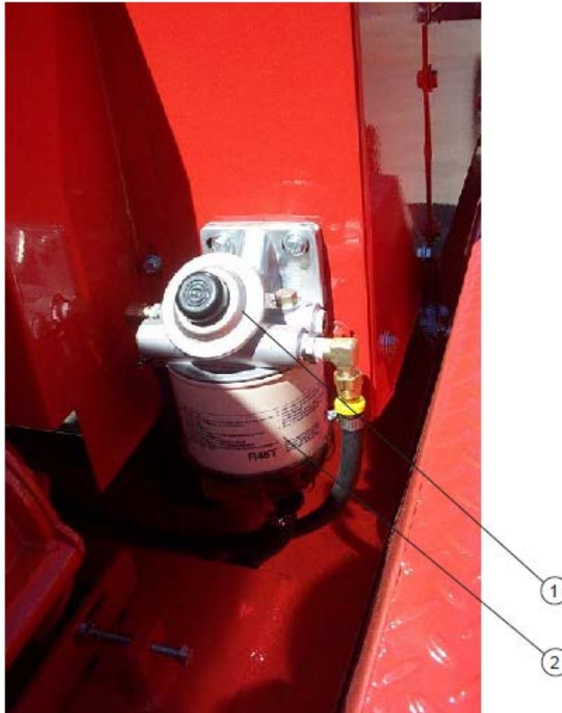
Figure 9.28 External Water/Fuel Separator Option
