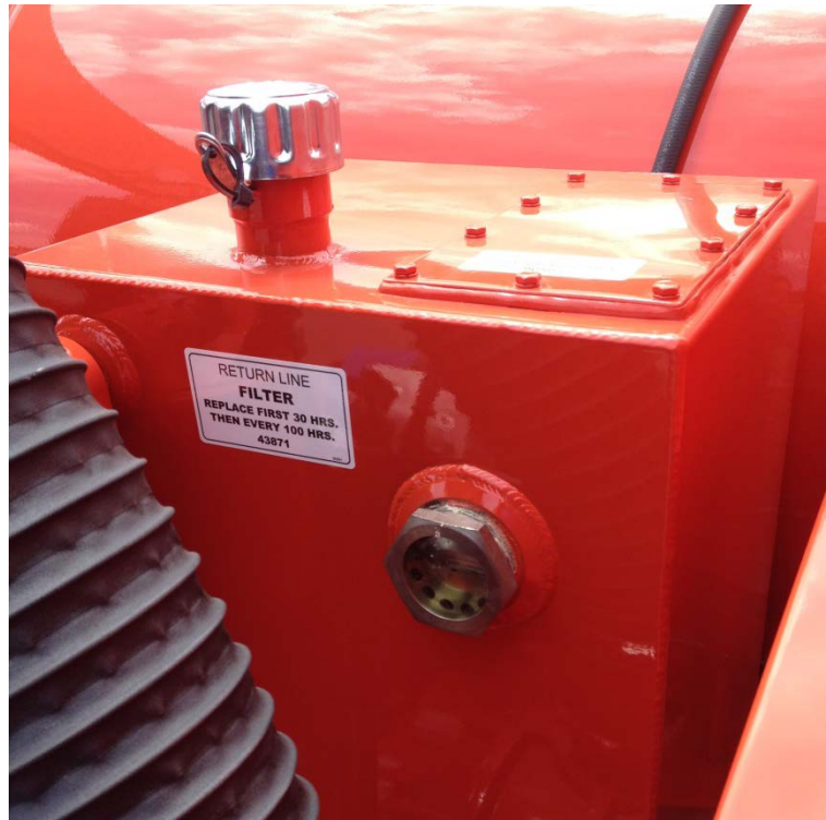
Figure 5.2 Hydraulic Fluid Fill Cap and Level Gauge
