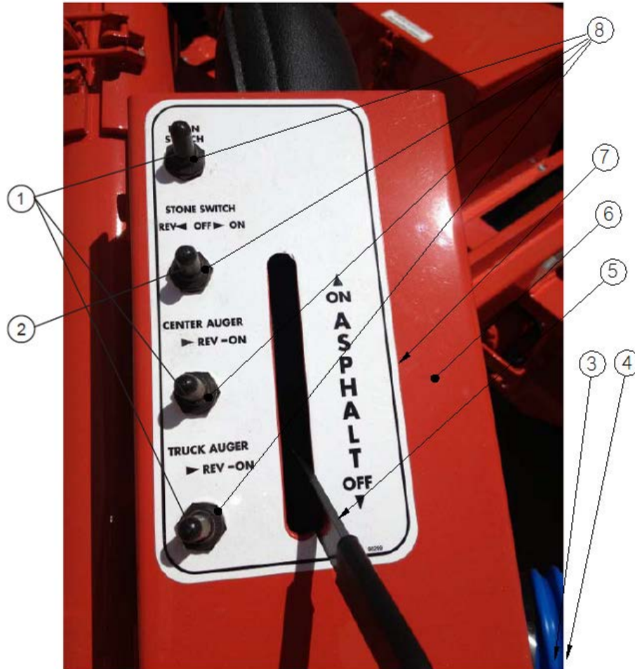
Figure 9.18 Boom Control Console
