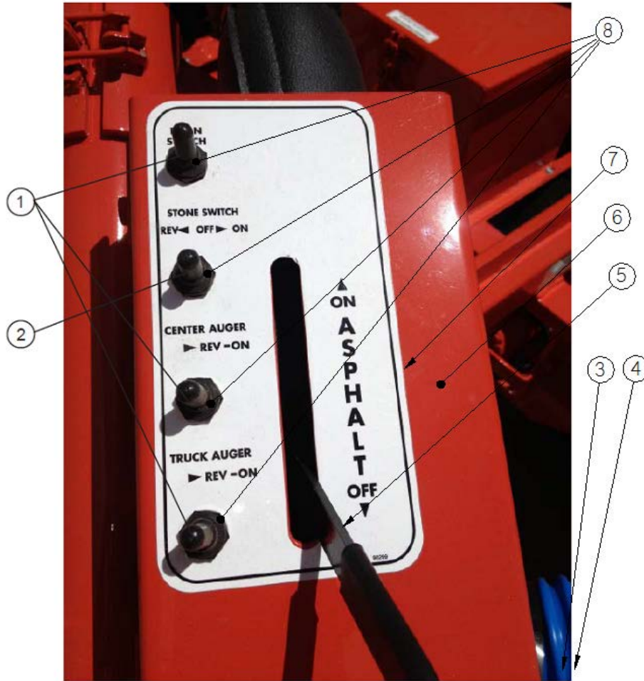
Figure 9.18 Boom Control Console
