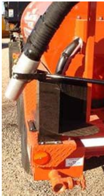
Figure 5.6 Nozzle Removed from Flush Box
