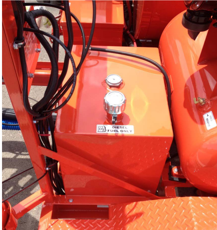
Figure 5.1 Diesel Fuel Fill Cap and Level Gauge
