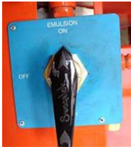
Figure 5.9 Emulsion Tank Valve
