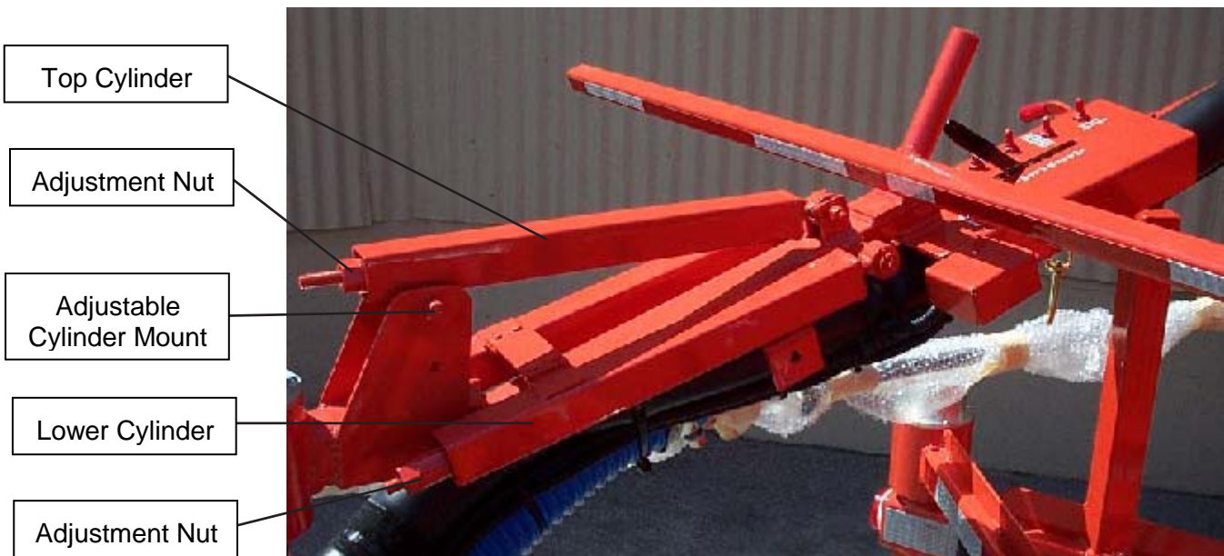
Figure 5.16 Boom Height Adjustment
