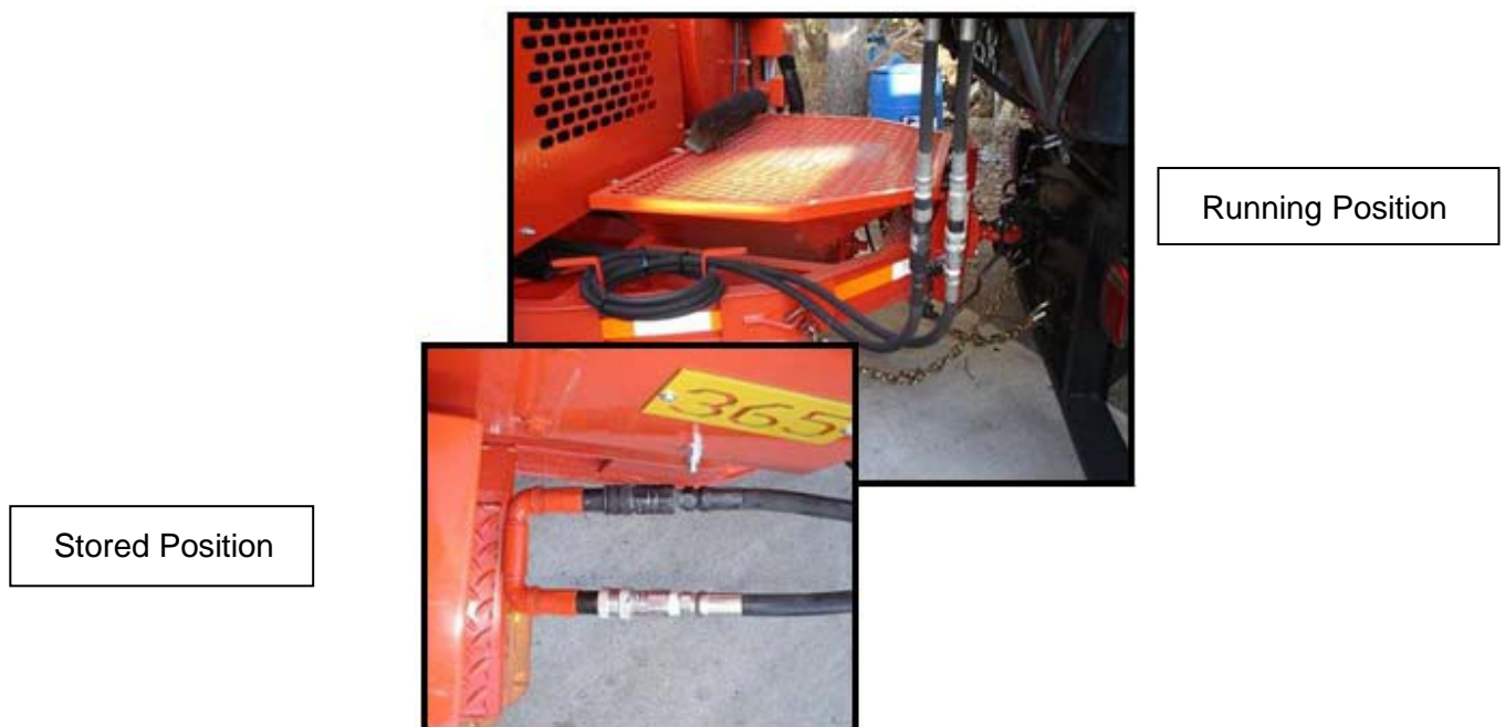
Figure 5.5 Tailgate Hydraulic Connections
