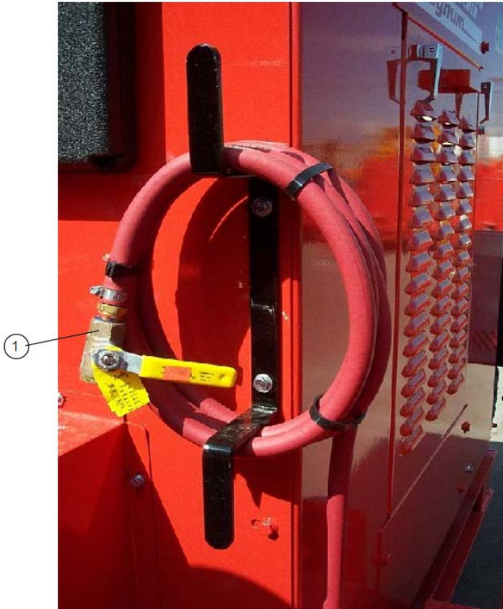
Figure 9.27 8 Foot Quick Flush Hose Option
