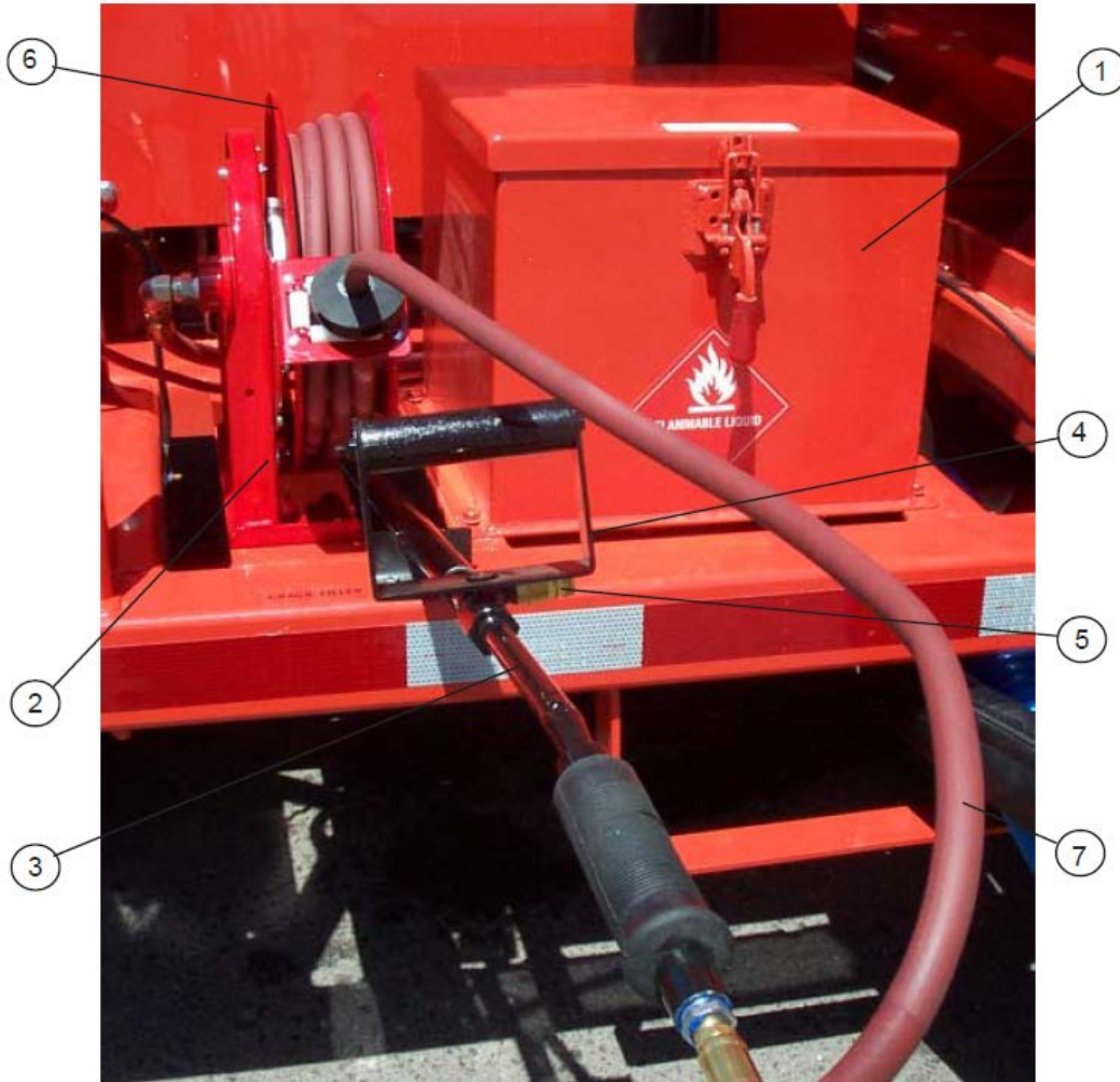
Figure 9.25 Crack Sealing Attachment
