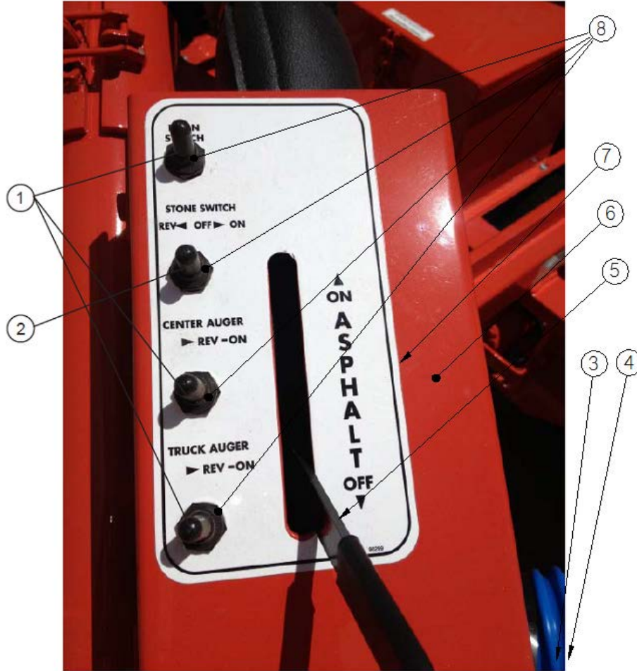
Figure 9.18 Boom Control Console
