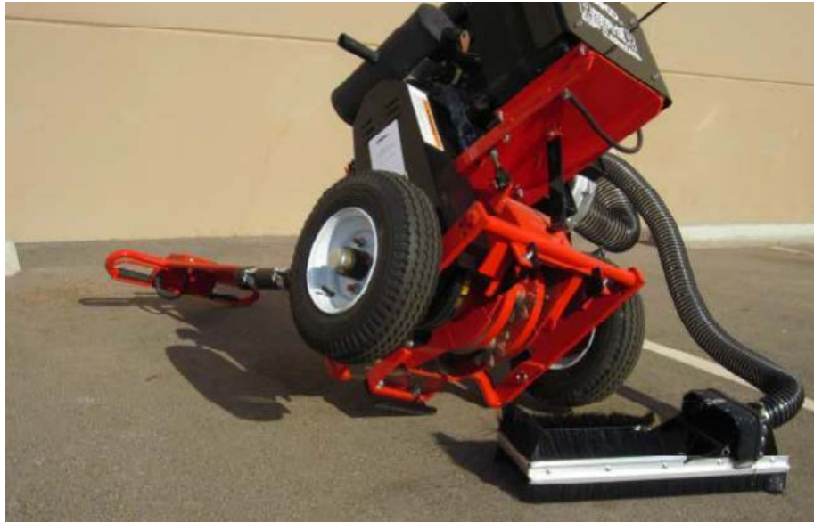
Figure 5.1 Model 30 Router Raised for Dust Shroud Installation
