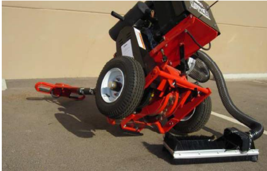
Figure 5-1 Model 30 Router Raised for Dust Shroud Installation
