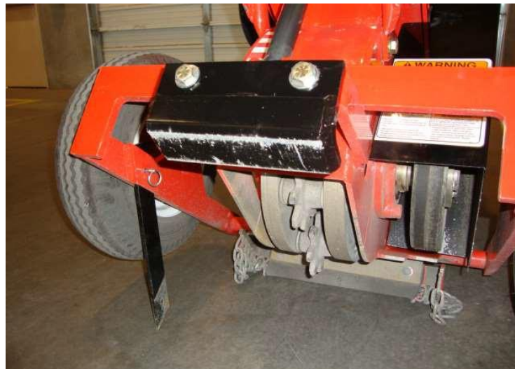
Figure 6-3 Raised Rear Support Strip
