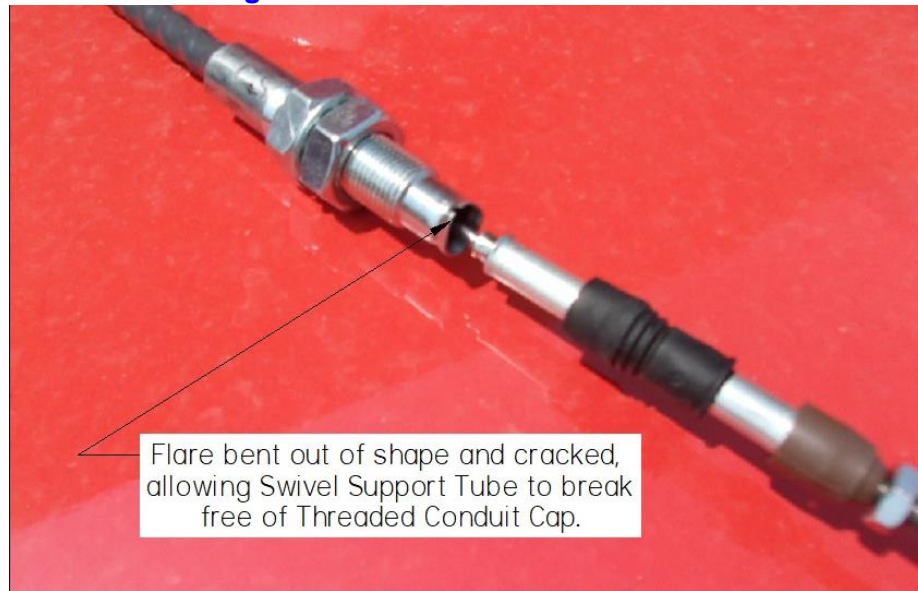
Figure 6-10 Broken Cable Reference
