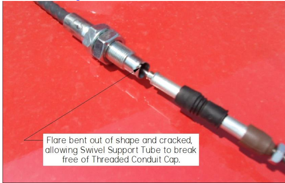
Figure 6-10 Broken Cable Reference
