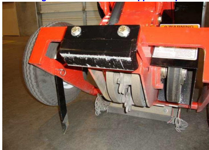
Figure 6-3 Raised Rear Support Strip
