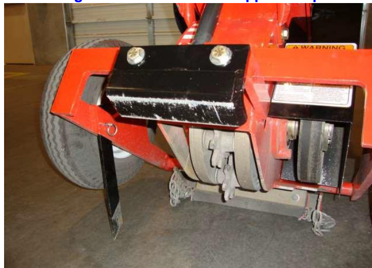
Figure 6-3 Raised Rear Support Strip
