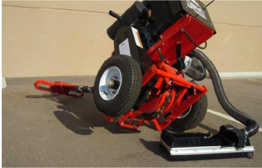
Figure 5-1 Model 30 Router Raised for Dust Shroud Installation
