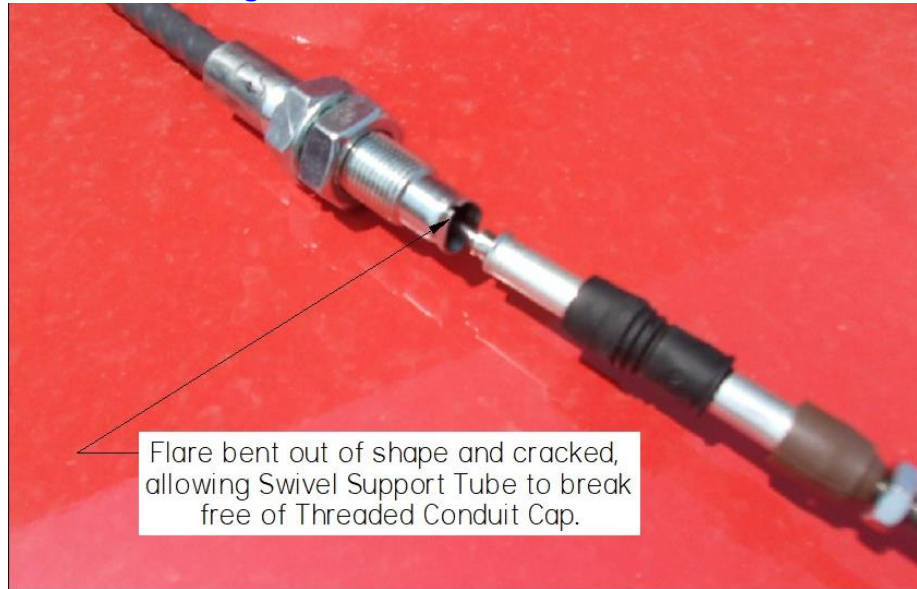
Figure 6-10 Broken Cable Reference
