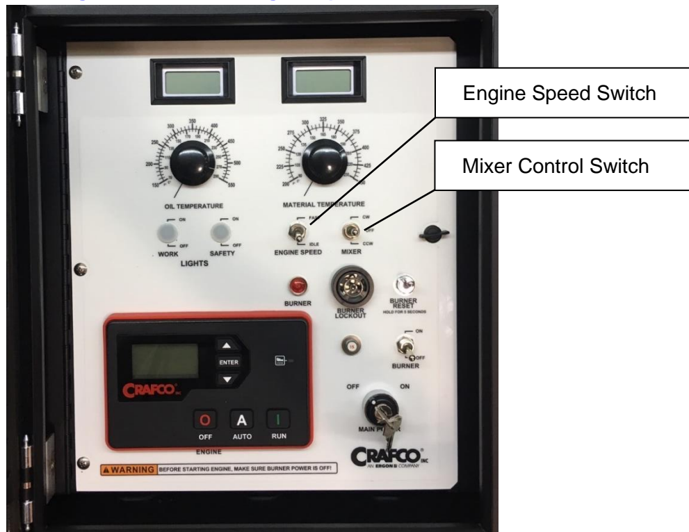
Figure 5-5 Mixer & Engine Speed Switch
