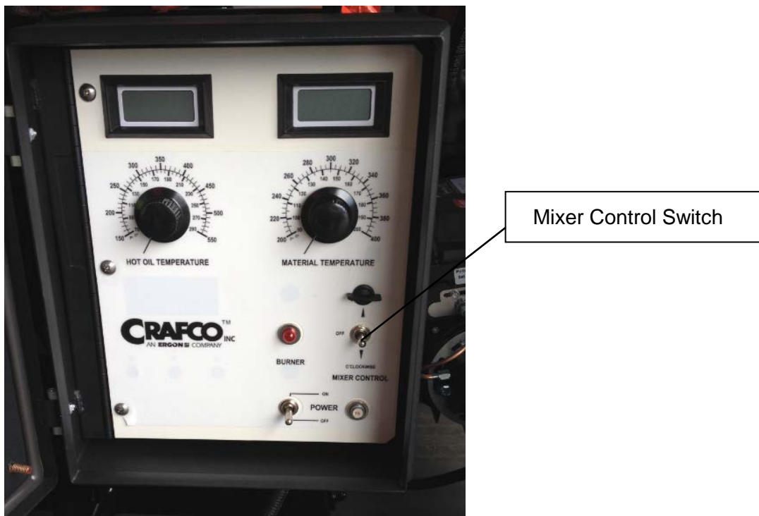
Figure 5-5 Mixer Control Switch
