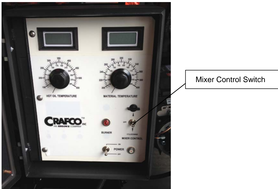
Figure 5-5 Mixer Control Switch
