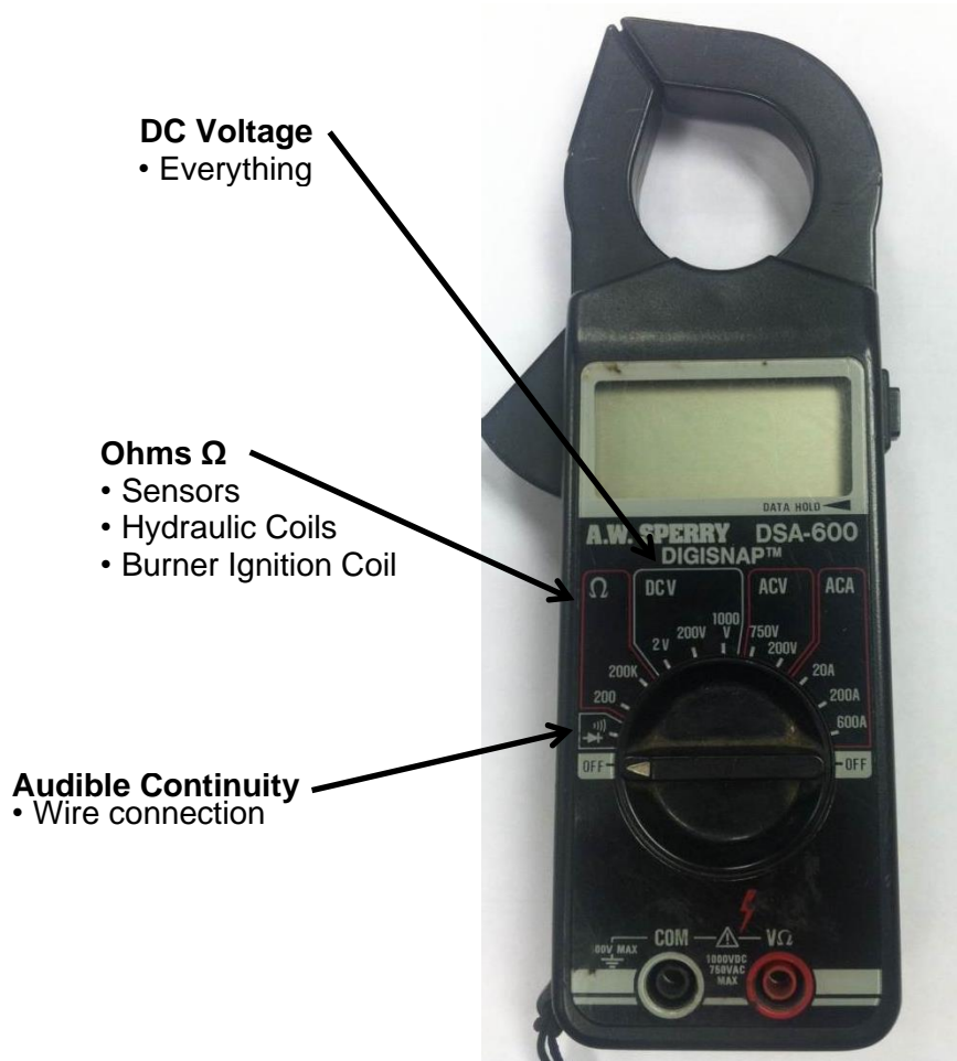
Figure 7-2 Clamp-On Amp Meter/Multimeter
