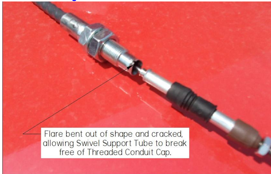
Figure 6-10 Broken Cable Reference
