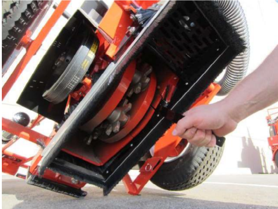
Figure 5-2 Using the Brush Manipulation Tool
