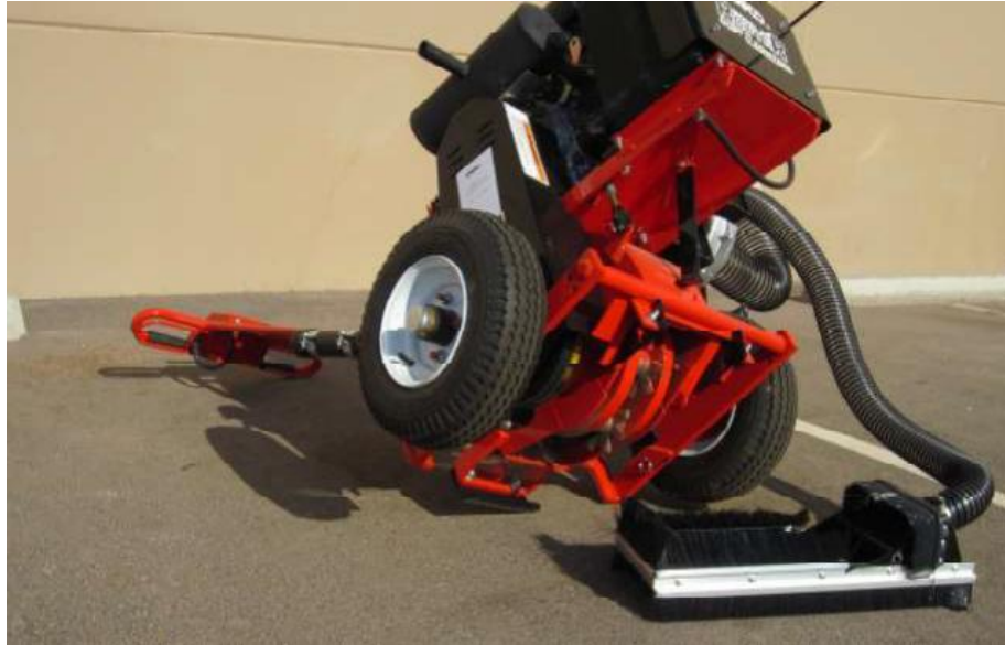
Figure 5-1 Model 30 Router Raised for Dust Shroud Installation
