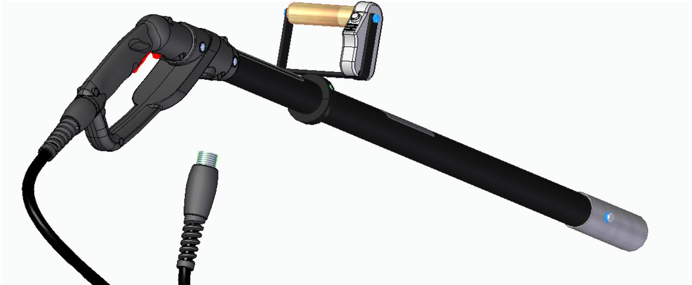
2. The handle is set up for a right-handed operator (right hand on rear handle/trigger, left hand on forward handle for horn). It can be switched by removing the bolt through the wooden dowel handle and transmitter, swapping positions (transmitter on left, dowel on right) and re-assembling.
