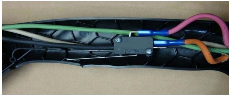
Fig. 6.4 Switch Wire Location
