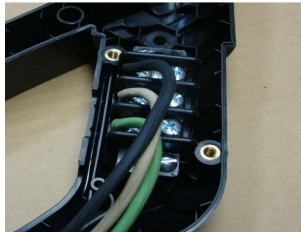
Fig. 6.6 Terminal Block Wiring
