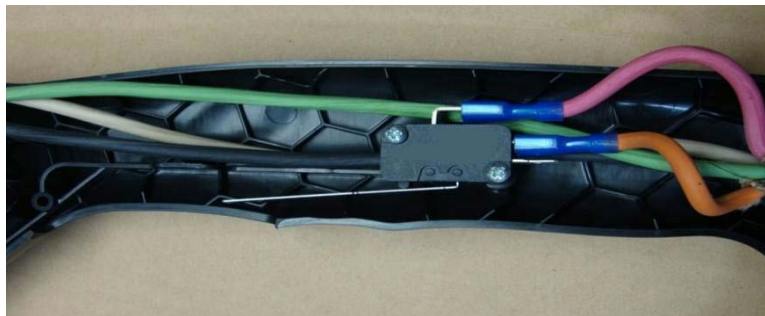
Fig. 6-4 Switch Wire Location
