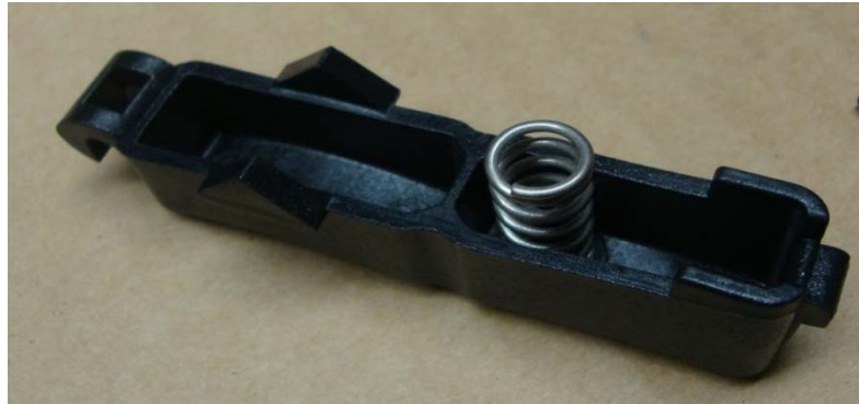
Fig. 6-7 Actuator Spring Location
