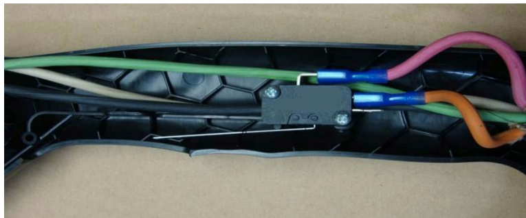
Fig. 6-4 Switch Wire Location
