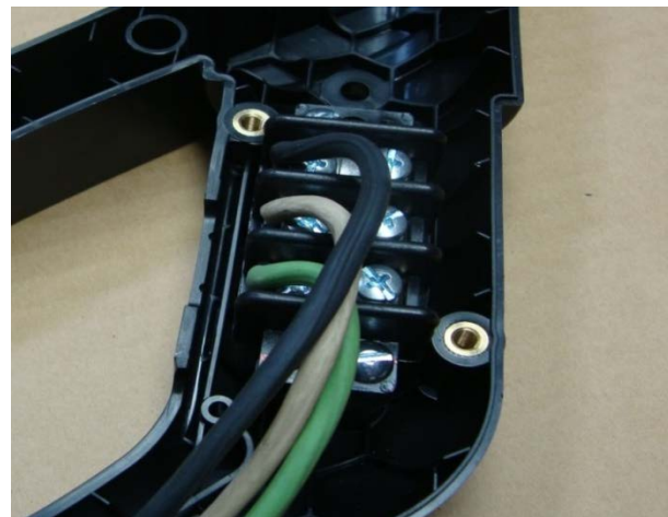
Fig. 6-5 Terminal Block Wiring
