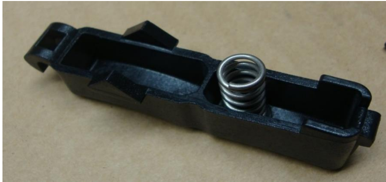
Fig. 6-8 Actuator Spring Location
