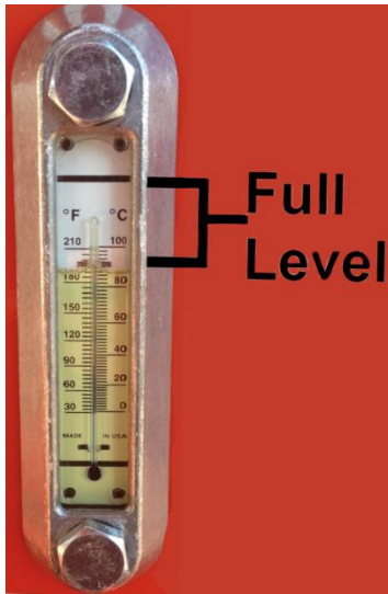
Fig. 5-1 Hydraulic Fluid Level and Temp. Gauge
