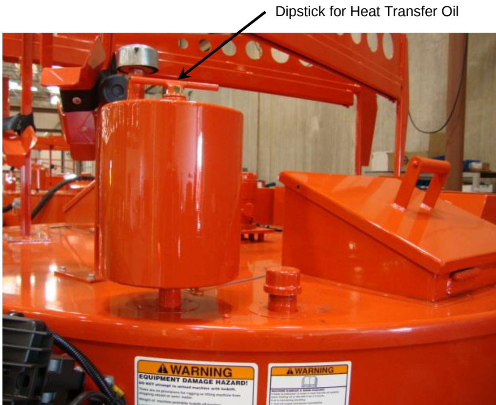
Fig. 5-3 Heat Transfer Oil Dipstick
