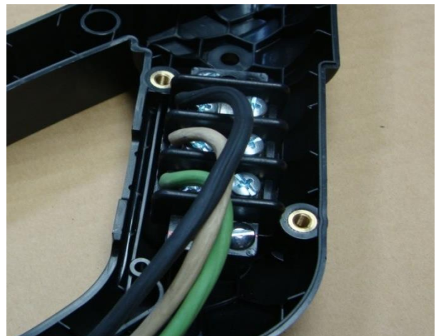
Fig. 6-6 Terminal Block Wiring
