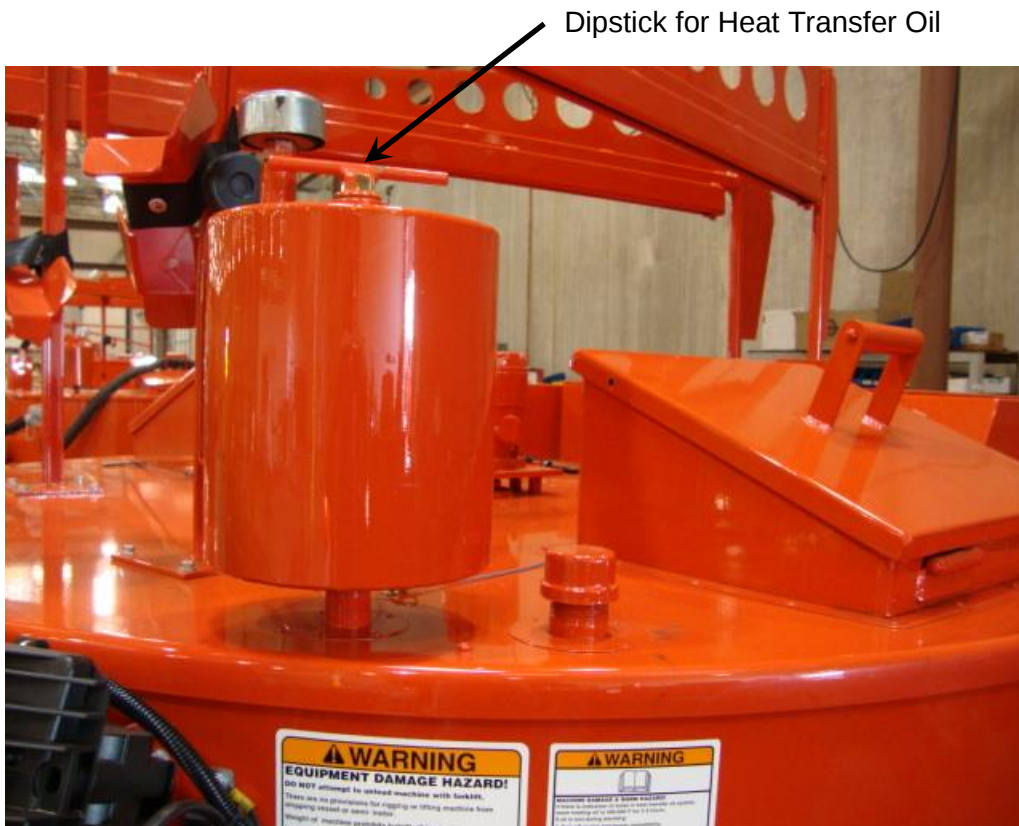
Fig. 5-3 Heat Transfer Oil Dipstick
