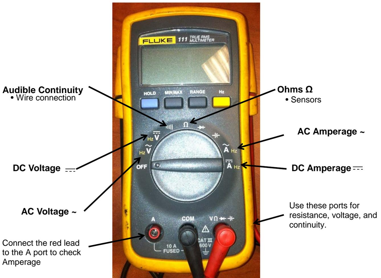
**Figure 7.1 Standard Multimeter**
