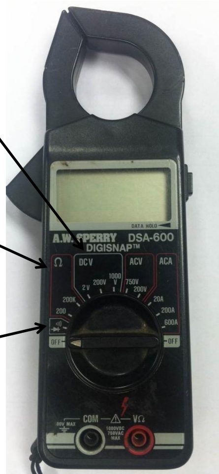
Figure 7-2 Clamp-On Amp Meter/Multimeter
