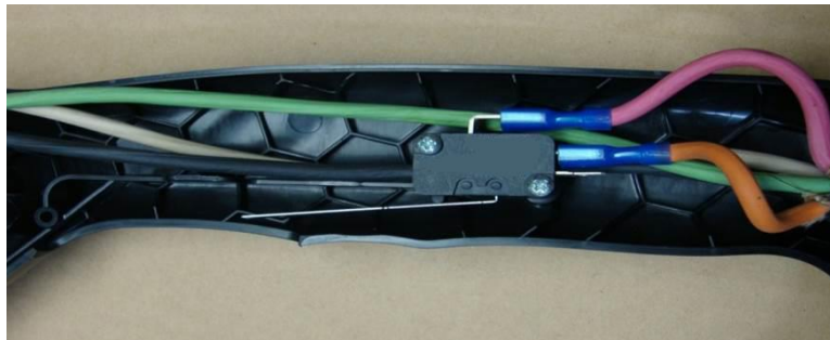
Fig. 6-15 Switch Wire Location
