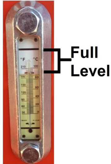
Fig. 5-1 Hydraulic Fluid Level and Temp. Gauge
