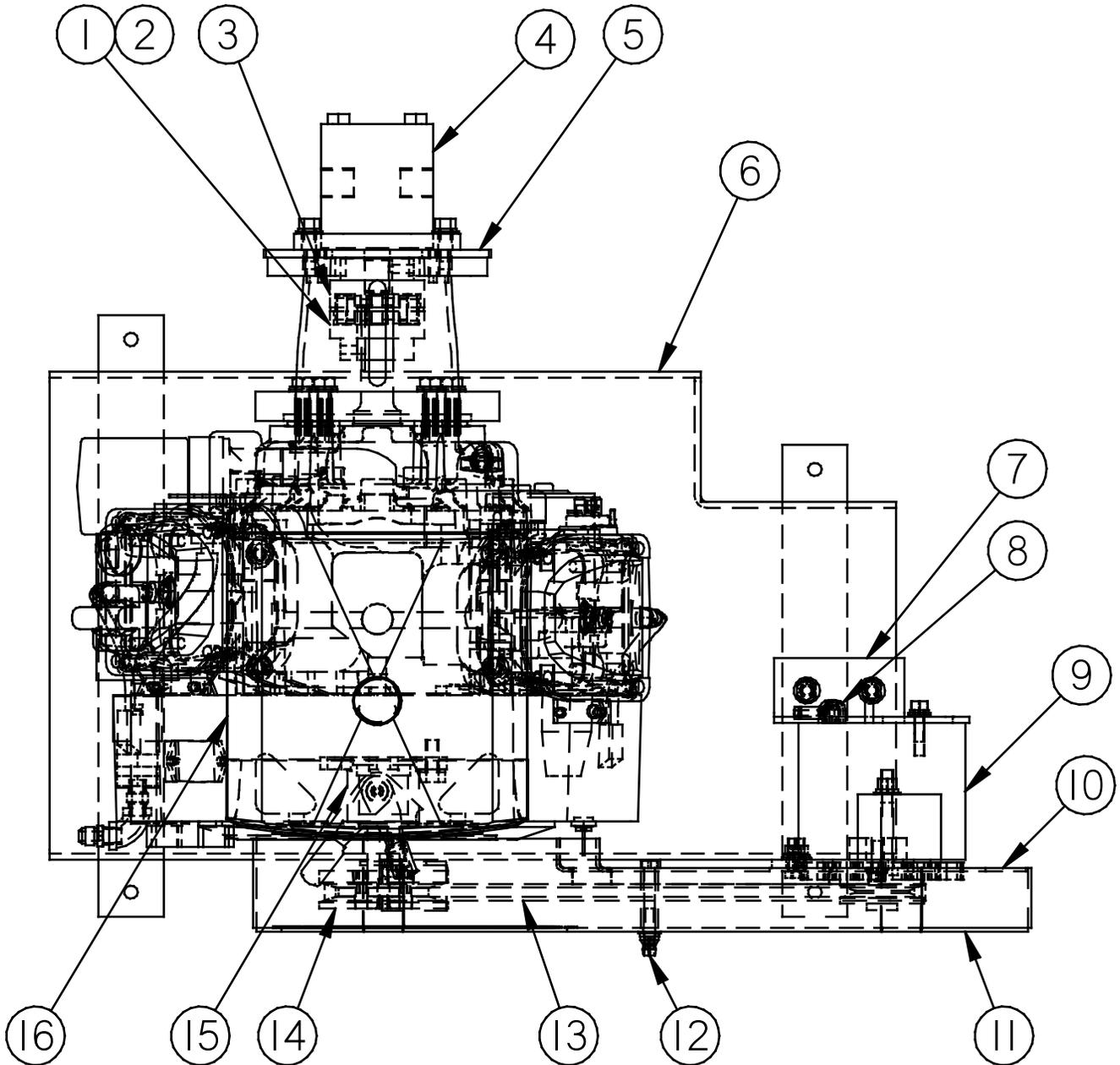
**Fig. 9-6 Engine Assembly: 44310**
