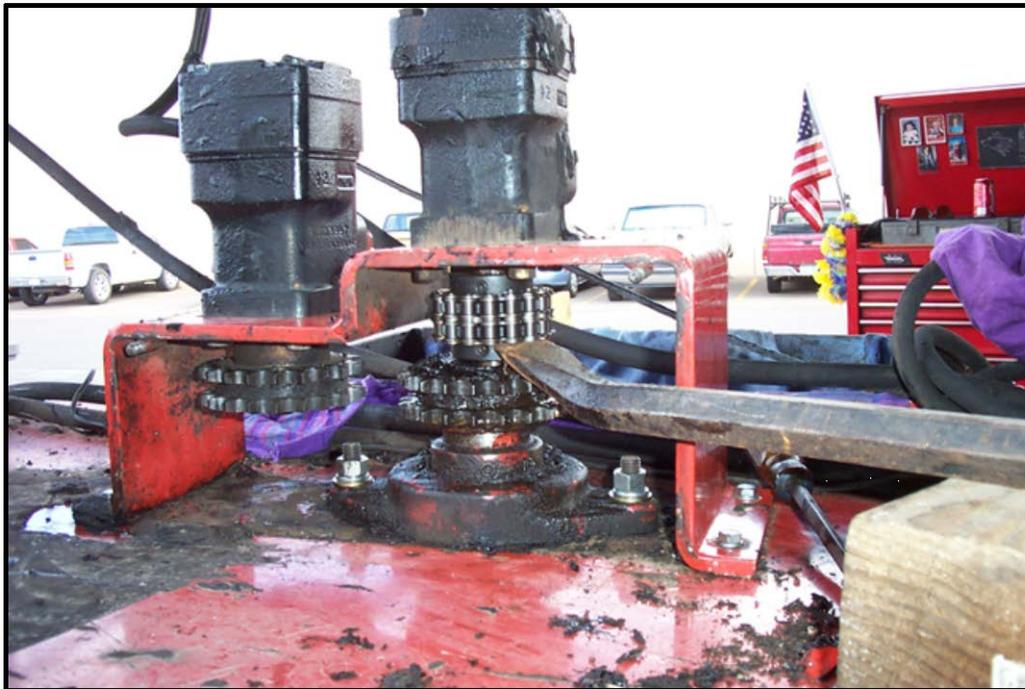
**Fig. 6-12 Pump Shaft to Hydraulic Pump Motor Placement**
