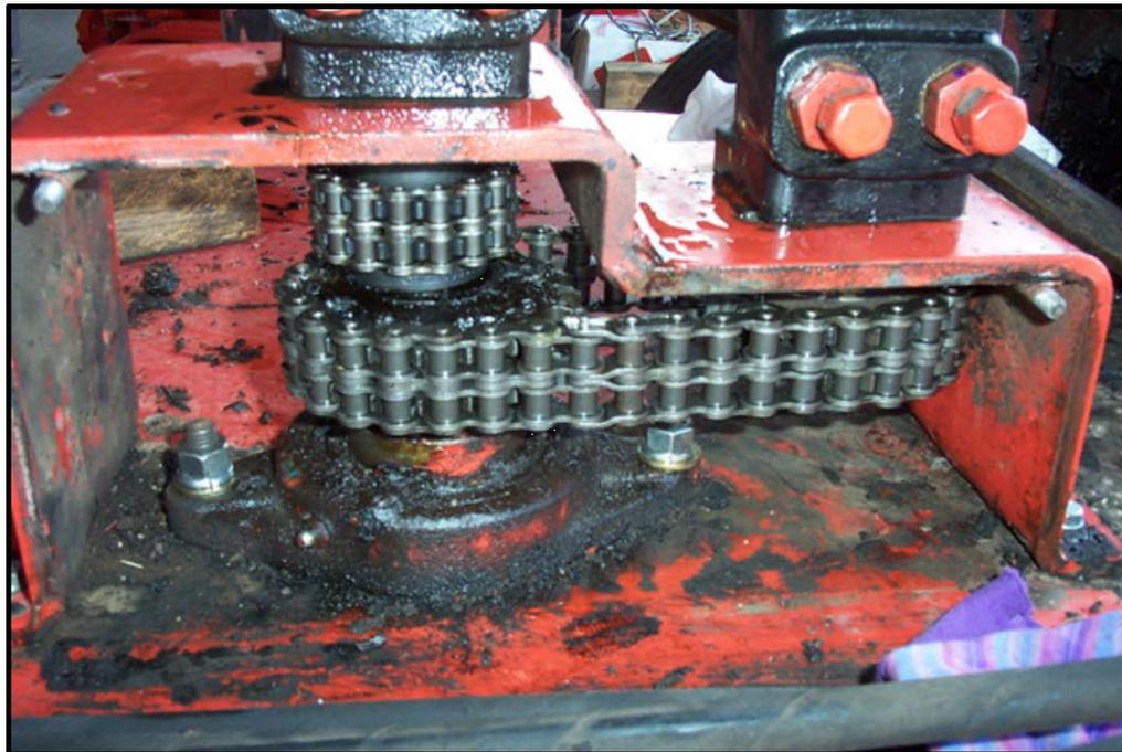
**Fig. 6-14 Agitator Chain Tightening Steps**
