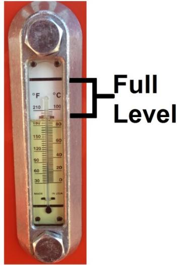
**Fig. 5-1 Hydraulic Fluid Level and Temp. Gauge**
