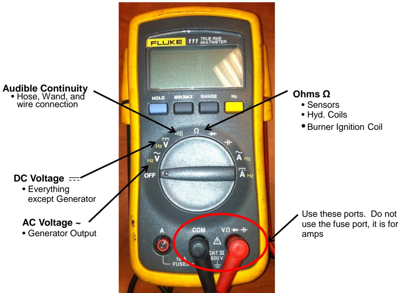
**Fig. 7-1 Standard Multimeter**
