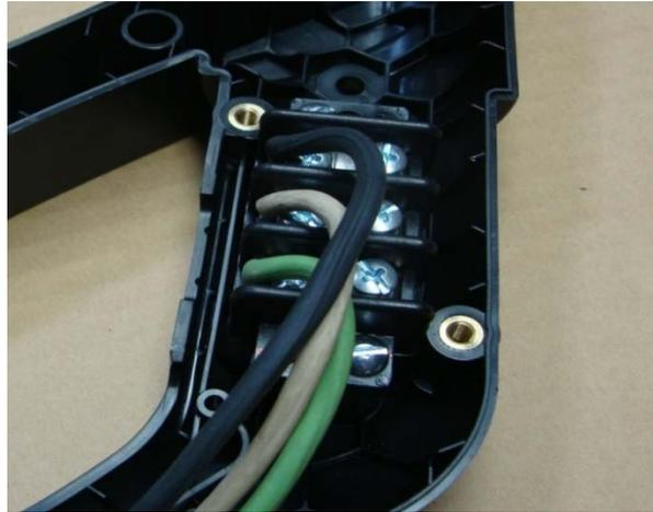
**Fig. 6-17 Terminal Block Wiring**
