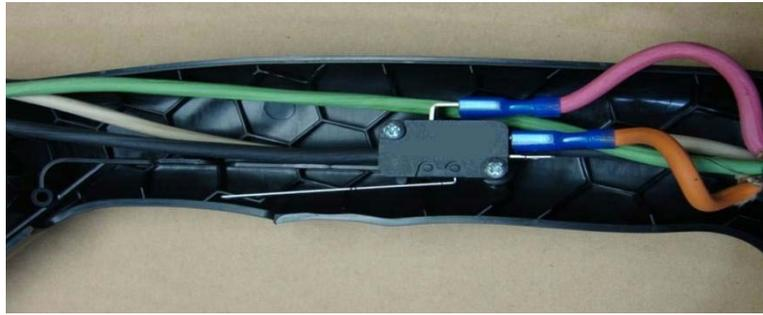
**Fig. 6-15 Switch Wire Location**
