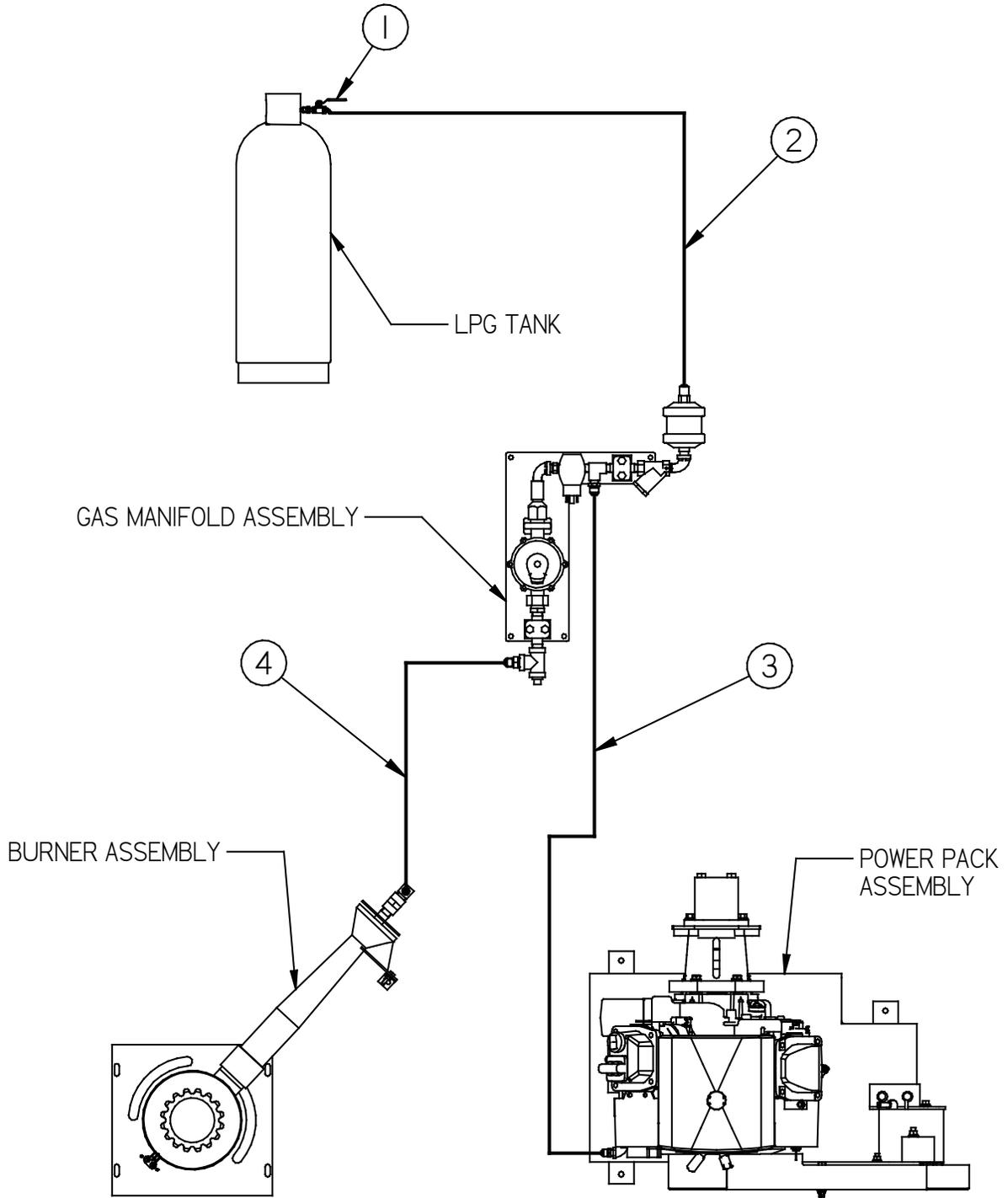
**Fig. 9-12 Propane Schematic**
