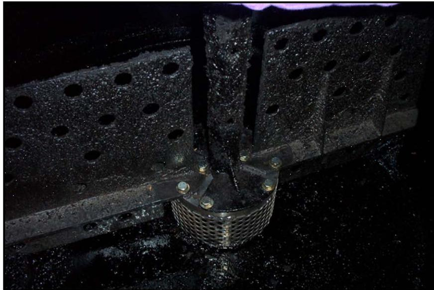
**Fig. 6-10 Agitator Shaft and Paddles Mounting**
