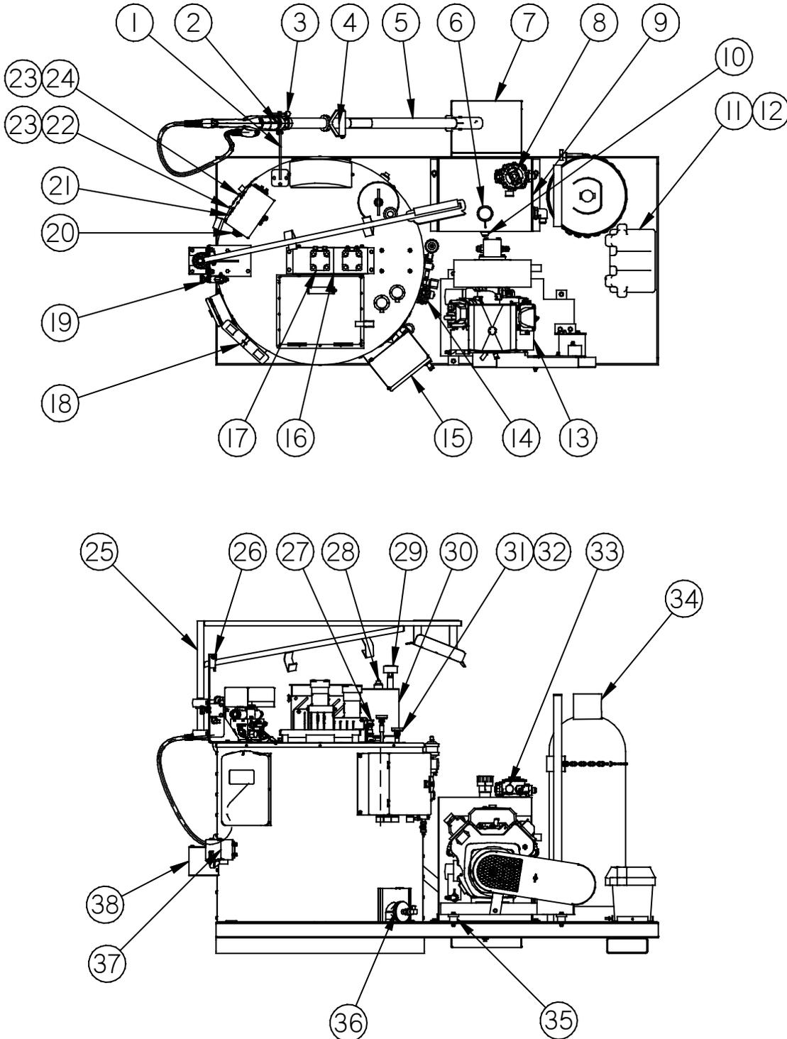
**Fig. 9-2 Super Shot 60 Propane Skid Melter: PN 50750**
