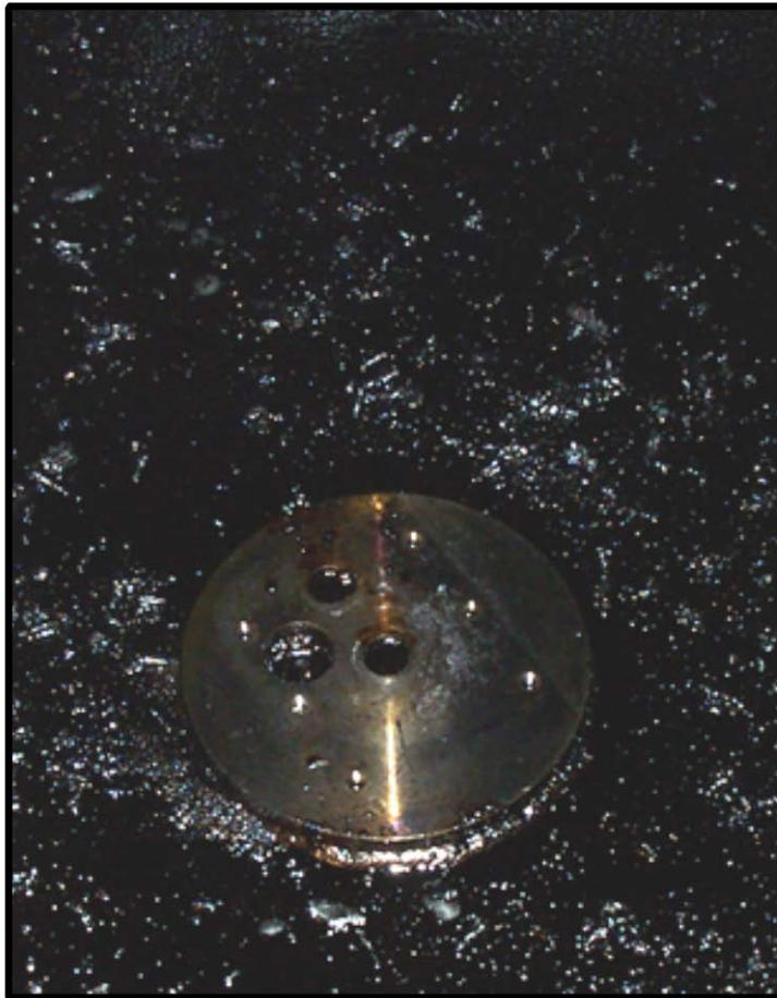
**Fig. 6-7 Cleaning of the Pump Mounting Plate**
