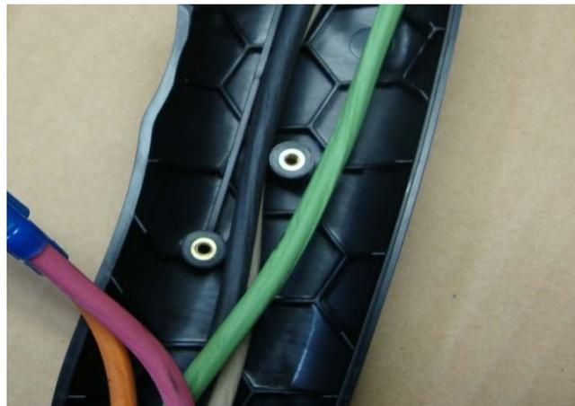
**Fig. 6-16 Wire Routing**
