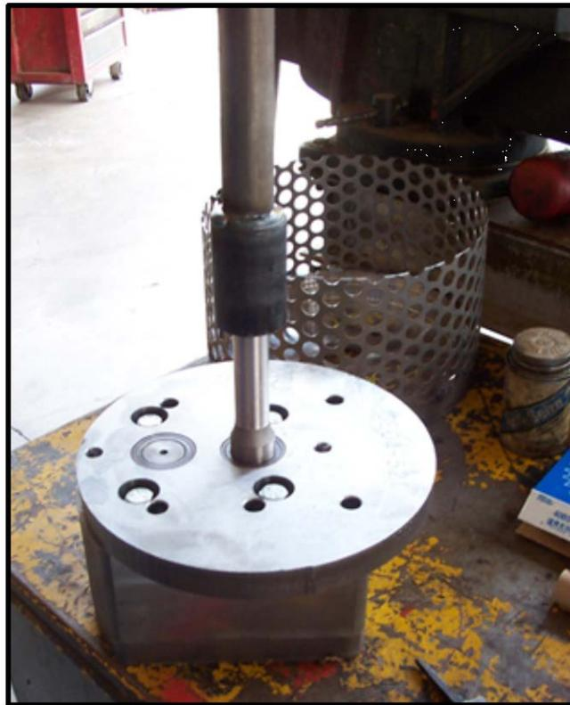
Fig. 6-8 Pump Drive Shaft Dry Fit to Material Pump
