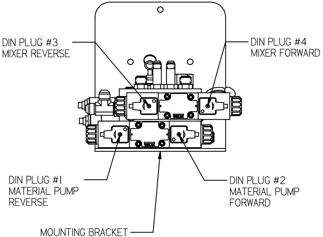
**Fig. 8-5 Din Plug Layout**
