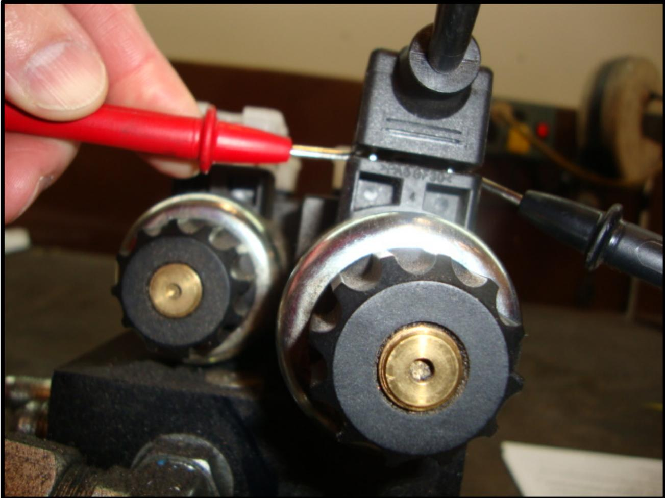
**Fig. 8-2 Checking Din Plug Voltage**
