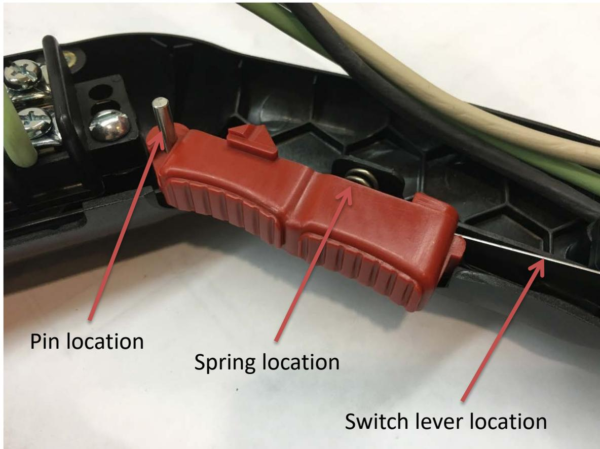
**Fig. 6-19 Actuator / Assembly**
