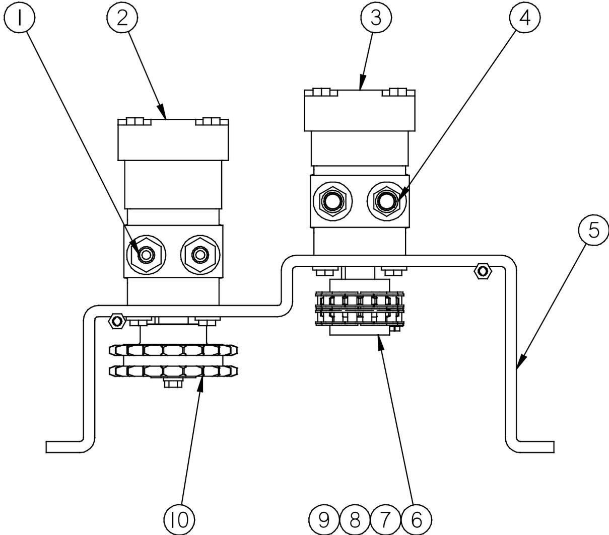
**Fig. 9-9 Pump/Mixer Motor Assembly: PN 44832**
