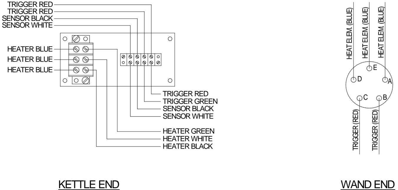
**Fig. 8-8 Junction Box Wiring**
