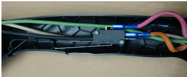
Fig. 6-16 Switch Wire Location
