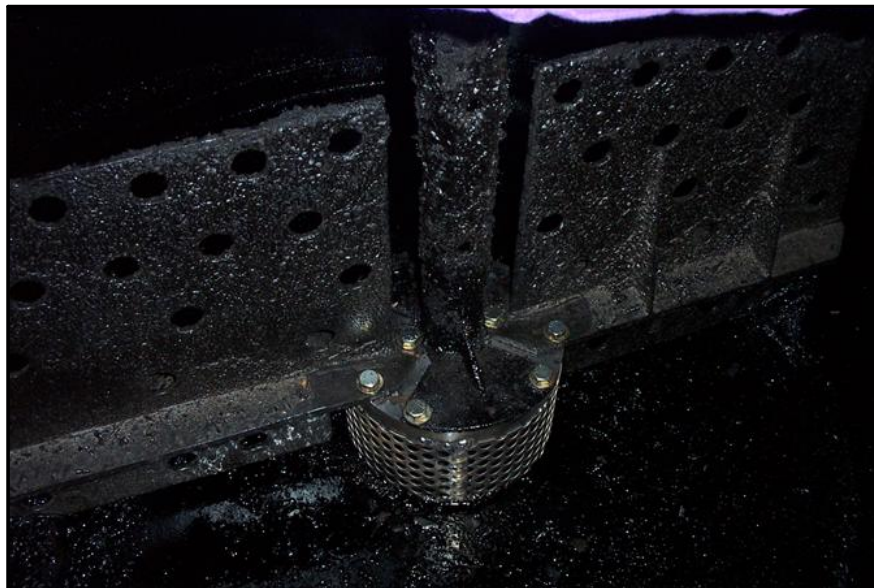
Fig. 6-11 Agitator Shaft and Paddles Mounting
