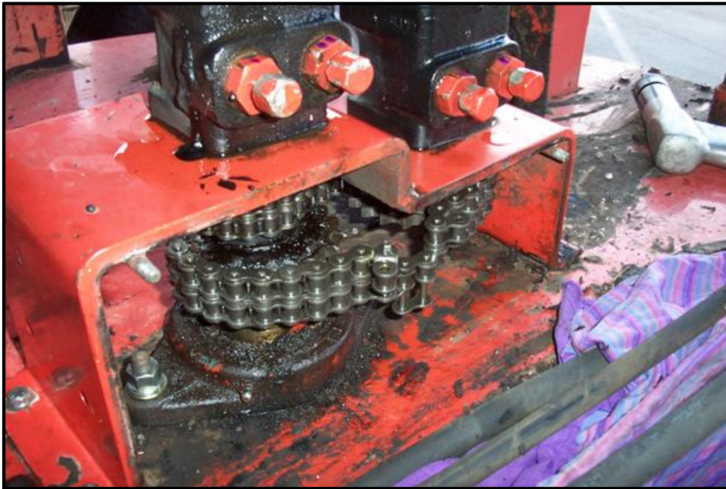
Fig. 6-14 Agitator Connecting Link
