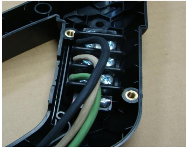
Fig. 6-18 Terminal Block Wiring
