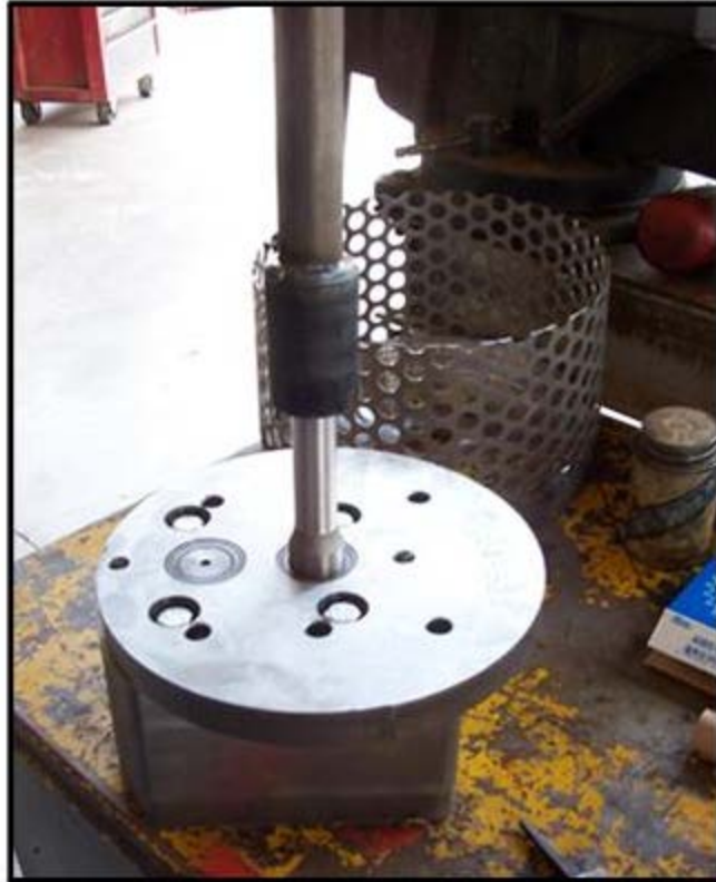
Figure 6.8 Pump Drive Shaft Dry Fit to Material Pump
