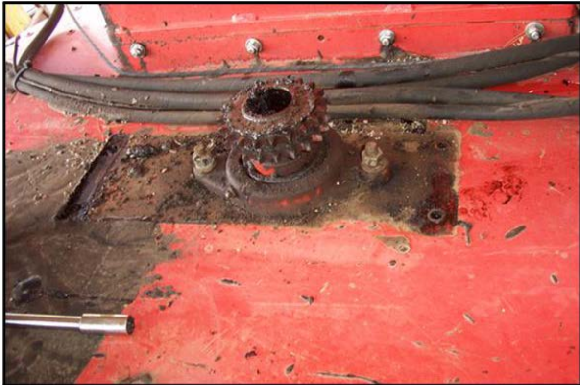
Figure 6.4 Removal of Motor Mount Assembly
