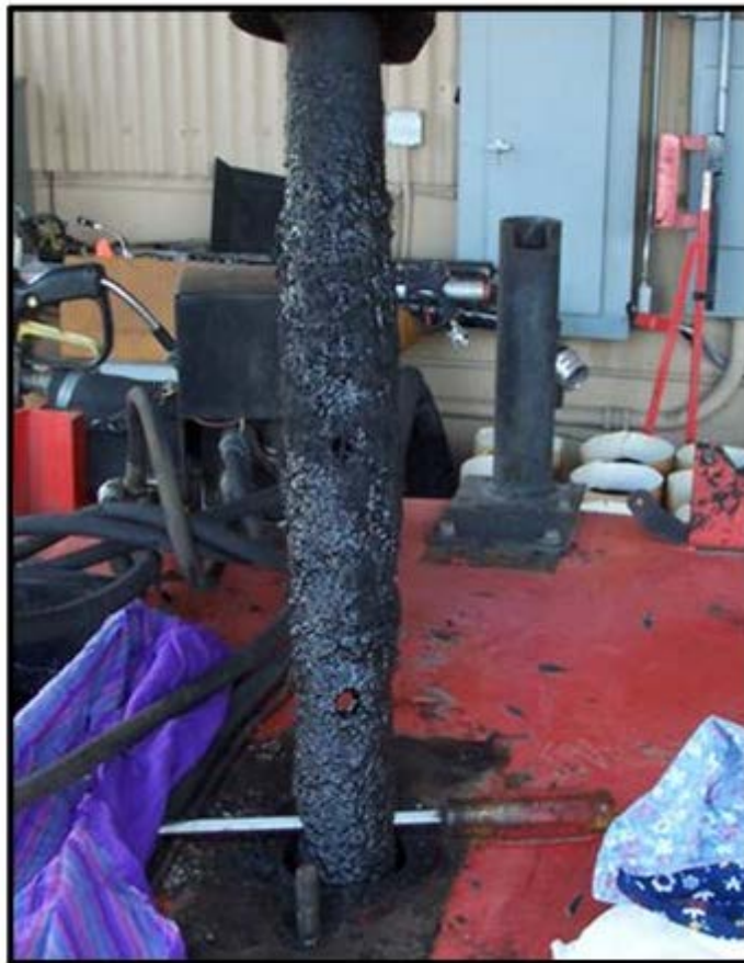
Figure 6.5 Supporting the Agitator Away from the Material Pump
