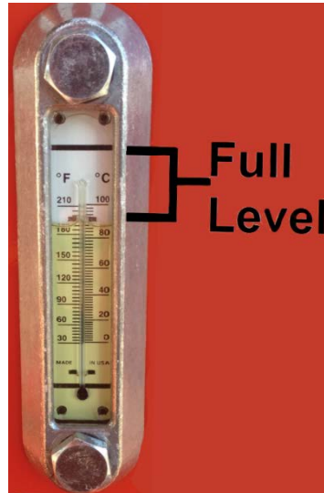
Figure 5.1 Hydraulic Fluid Level and Temp. Gauge
