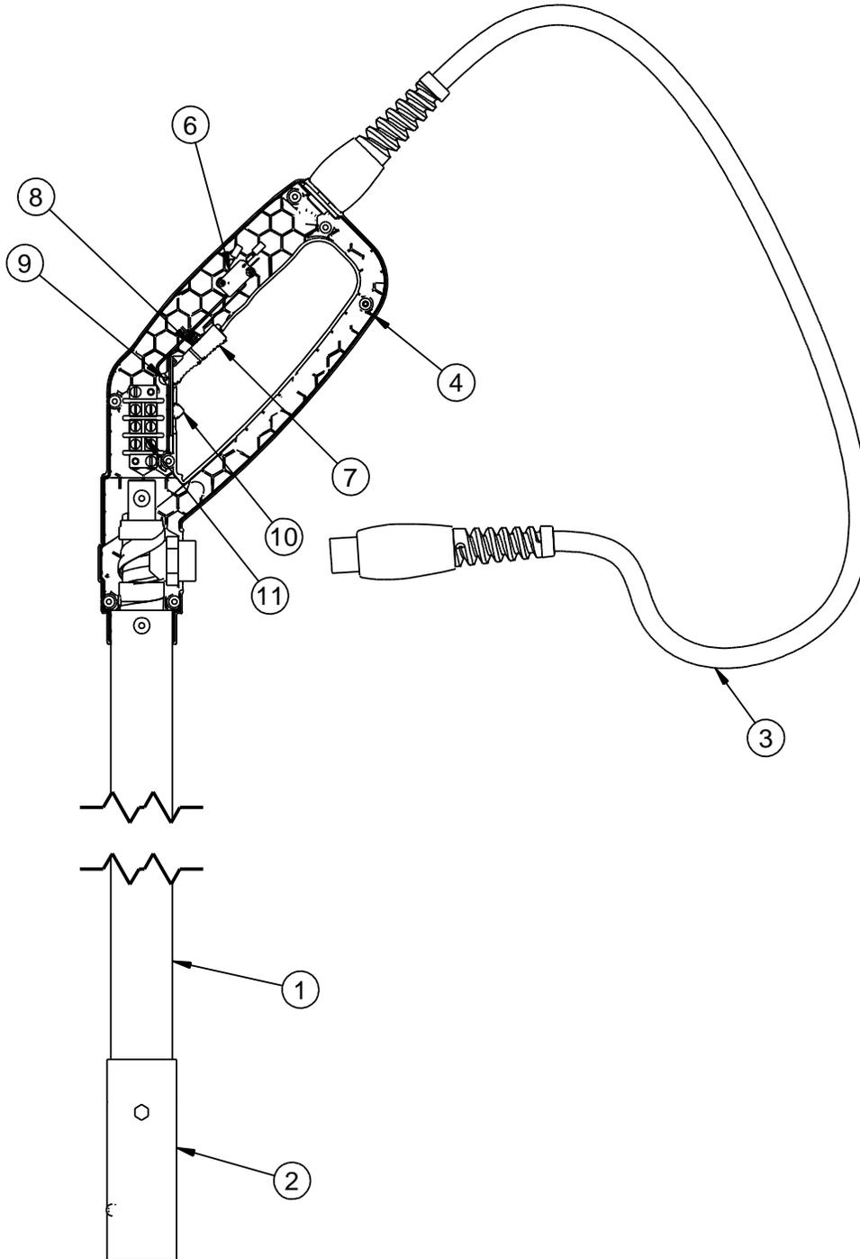
**Fig. 9-19 Wand Assembly: PN 52200 All Models**
