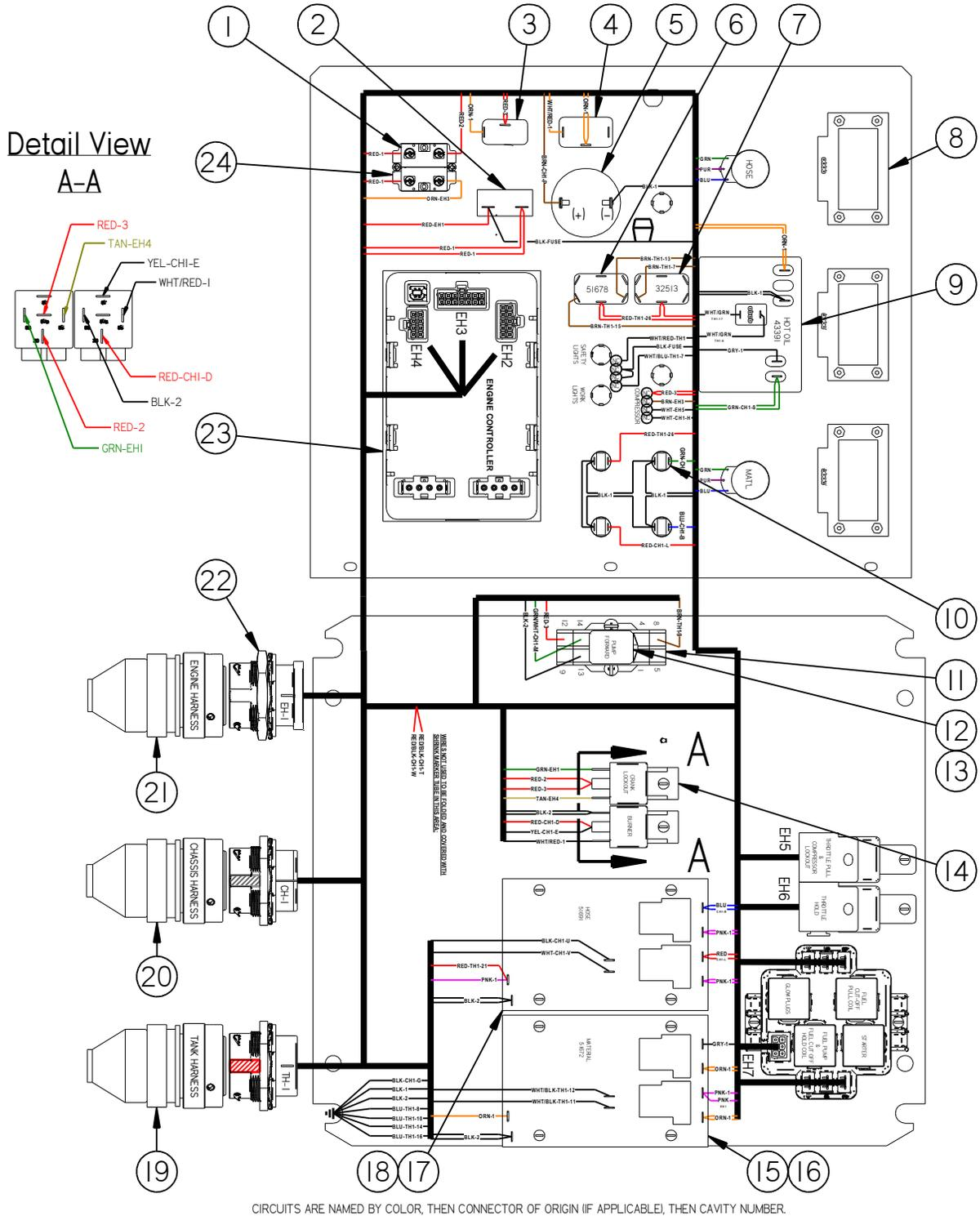
**Fig. 9-8 Control Box Assembly: PN 47250N All Models**
