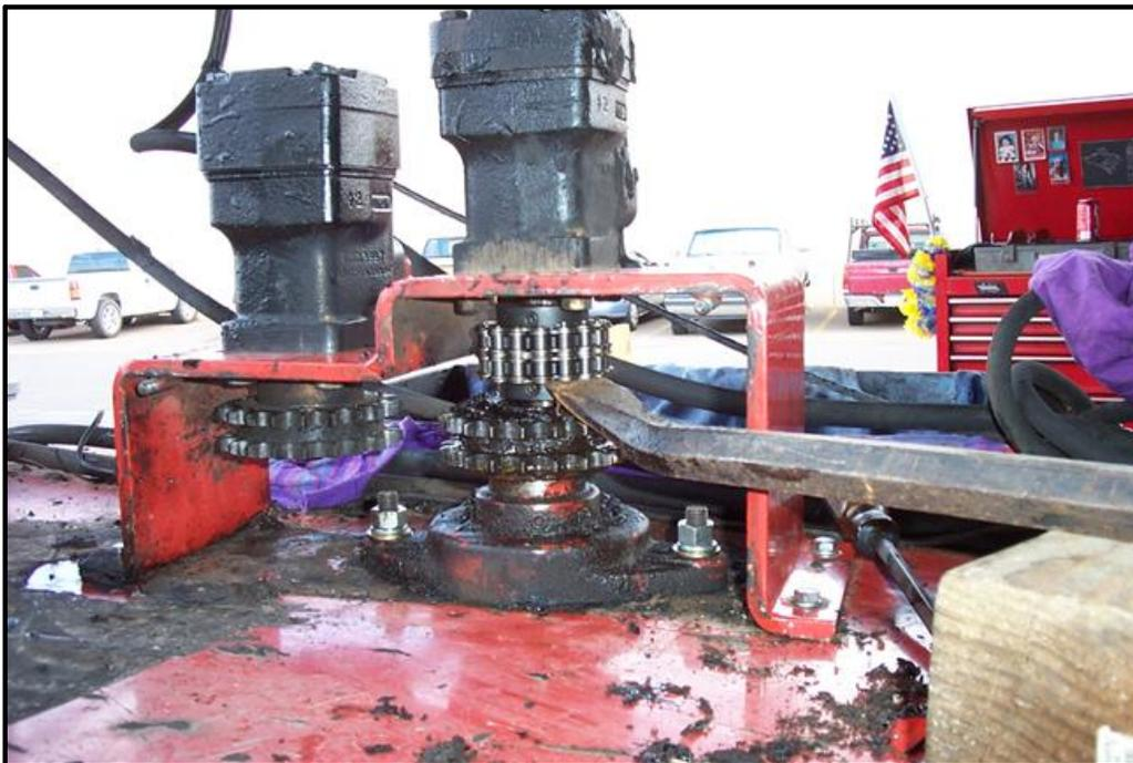
**Fig. 6-13 Pump Shaft to Hydraulic Pump Motor Placement**
