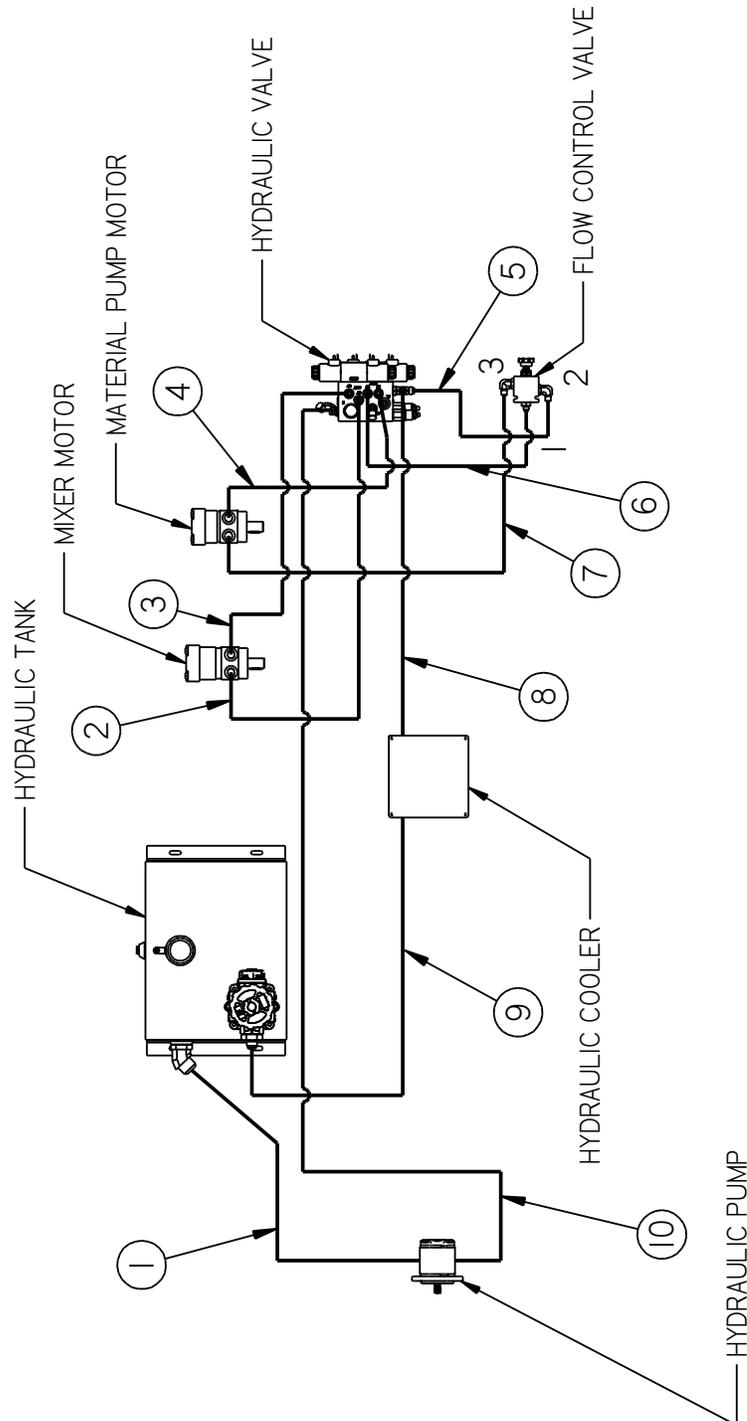
**Fig. 9-14 Hydraulic Diagram: PN 26669N (58700N & 58750N)**
