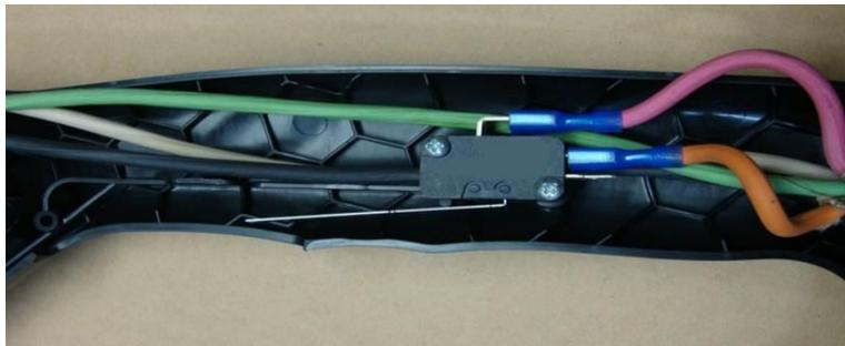
**Fig. 6-17 Switch Wire Location**
