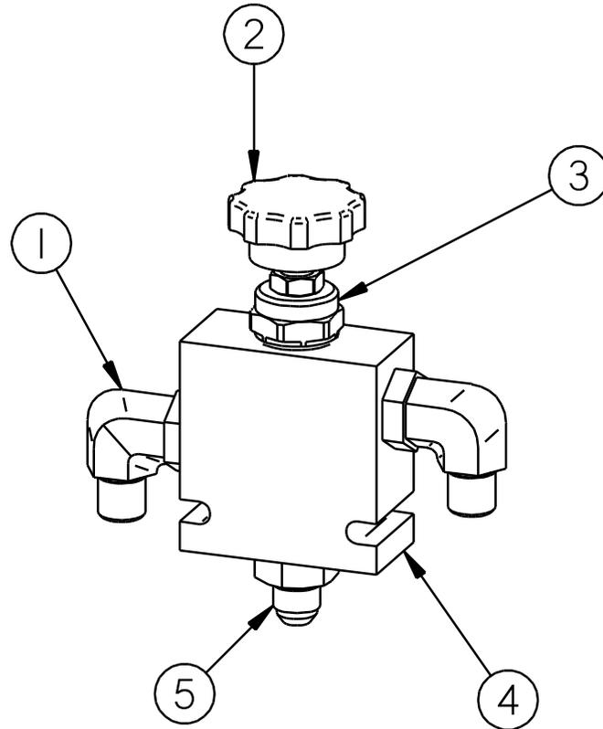
**Fig. 9-11 Material Flow Control Assembly: PN 46060 All Models**
