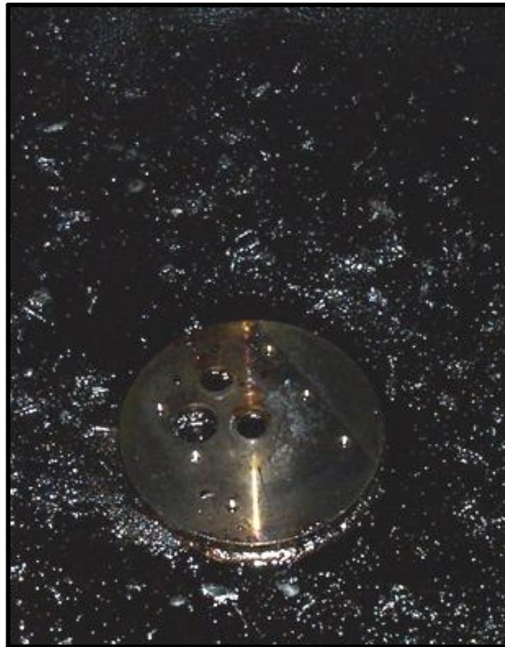
**Fig. 6-8 Cleaning of the Pump Mounting Plate**
