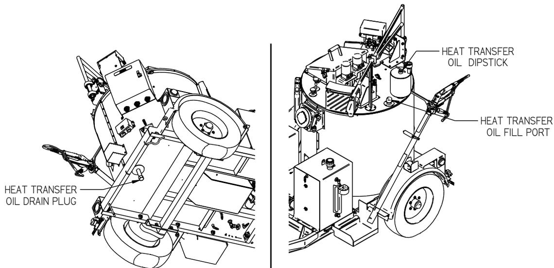
**Fig. 6-3 Heat Transfer Oil Drain and Fill Ports**
