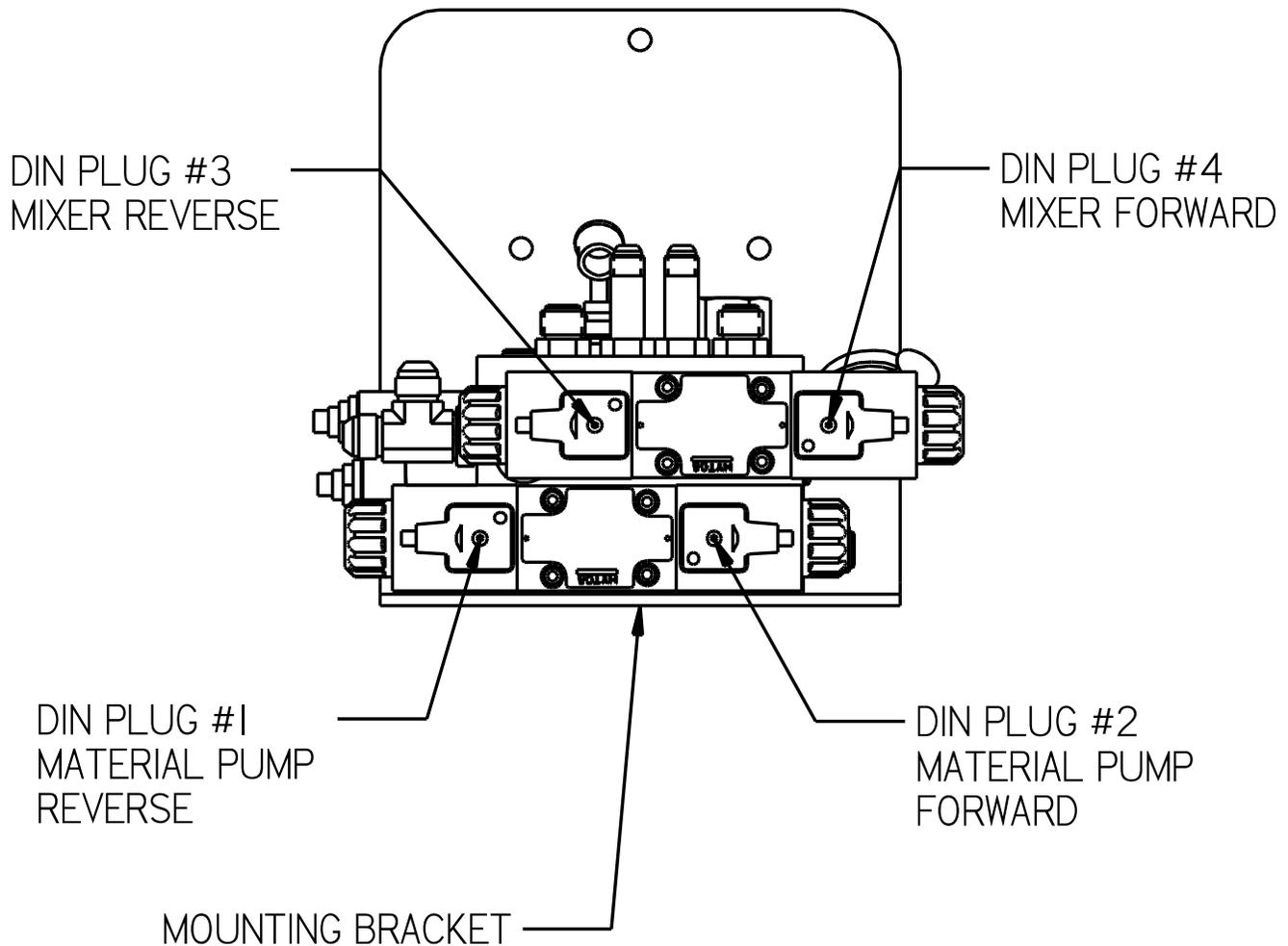
**Fig. 8-7 Din Plug Layout**
