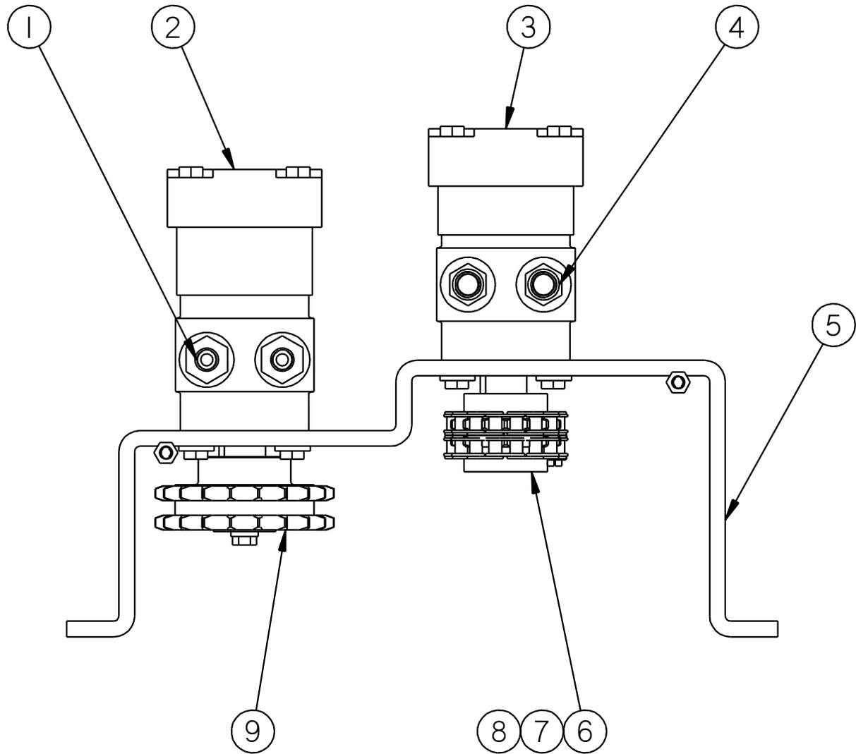
**Fig. 9-12 Pump/Mixer Motor Assembly: PN 44832 All Models**
