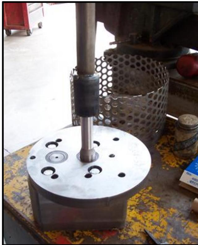
Fig. 6-9 Pump Drive Shaft Dry Fit to Material Pump
