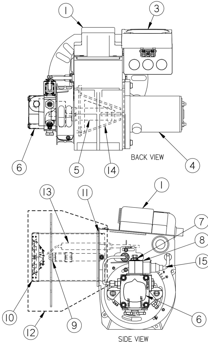
**Fig. 9-13 Diesel Burner Assembly: PN 46380 All Models**
