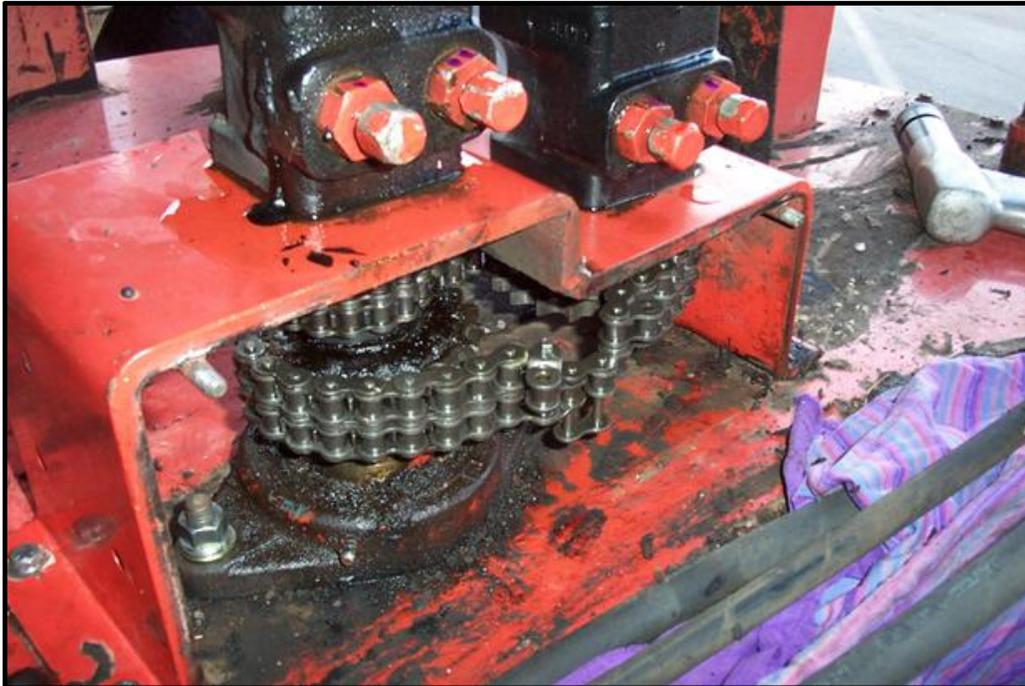
**Fig. 6-14 Agitator Connecting Link**
