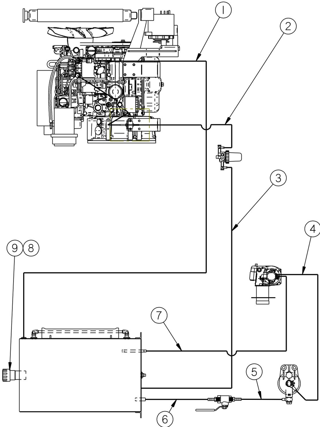
**Fig. 9-16 Diesel Fuel Line Schematic (58700N & 58750N)**
