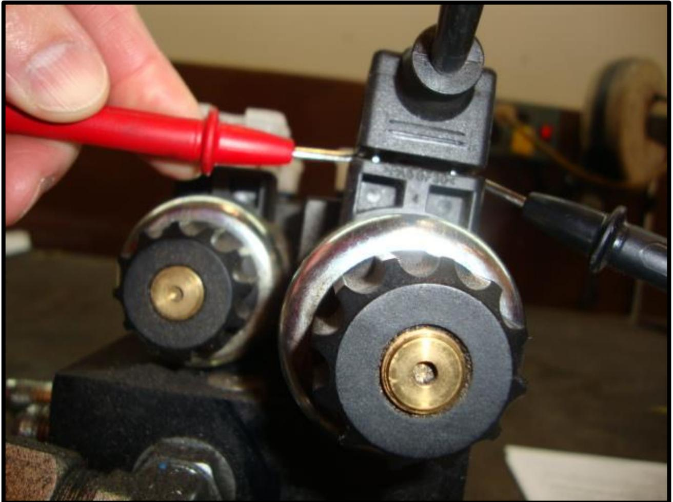
**Fig. 8-4 Checking Din Plug Voltage**
