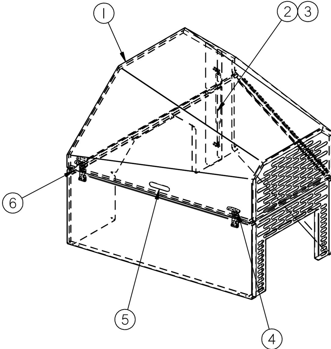
**Fig. 9-21 Optional Engine Cover for 3CH1 Engine All Models**
