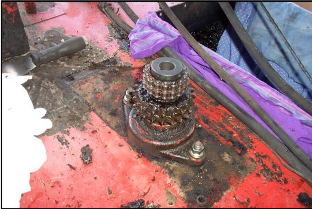
**Fig. 6-12 Pump Shaft Placement**
