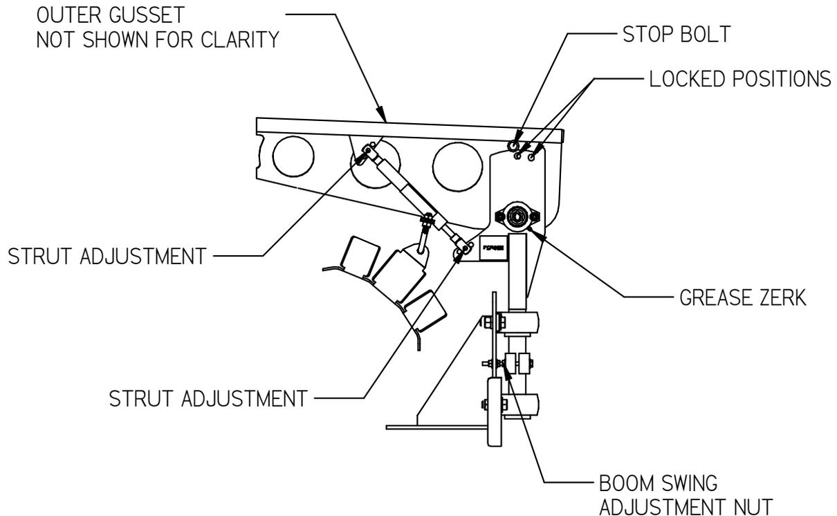
**Fig. 6-16 Flex Boom Adjustment****6.21.1 Strut Adjustment**
