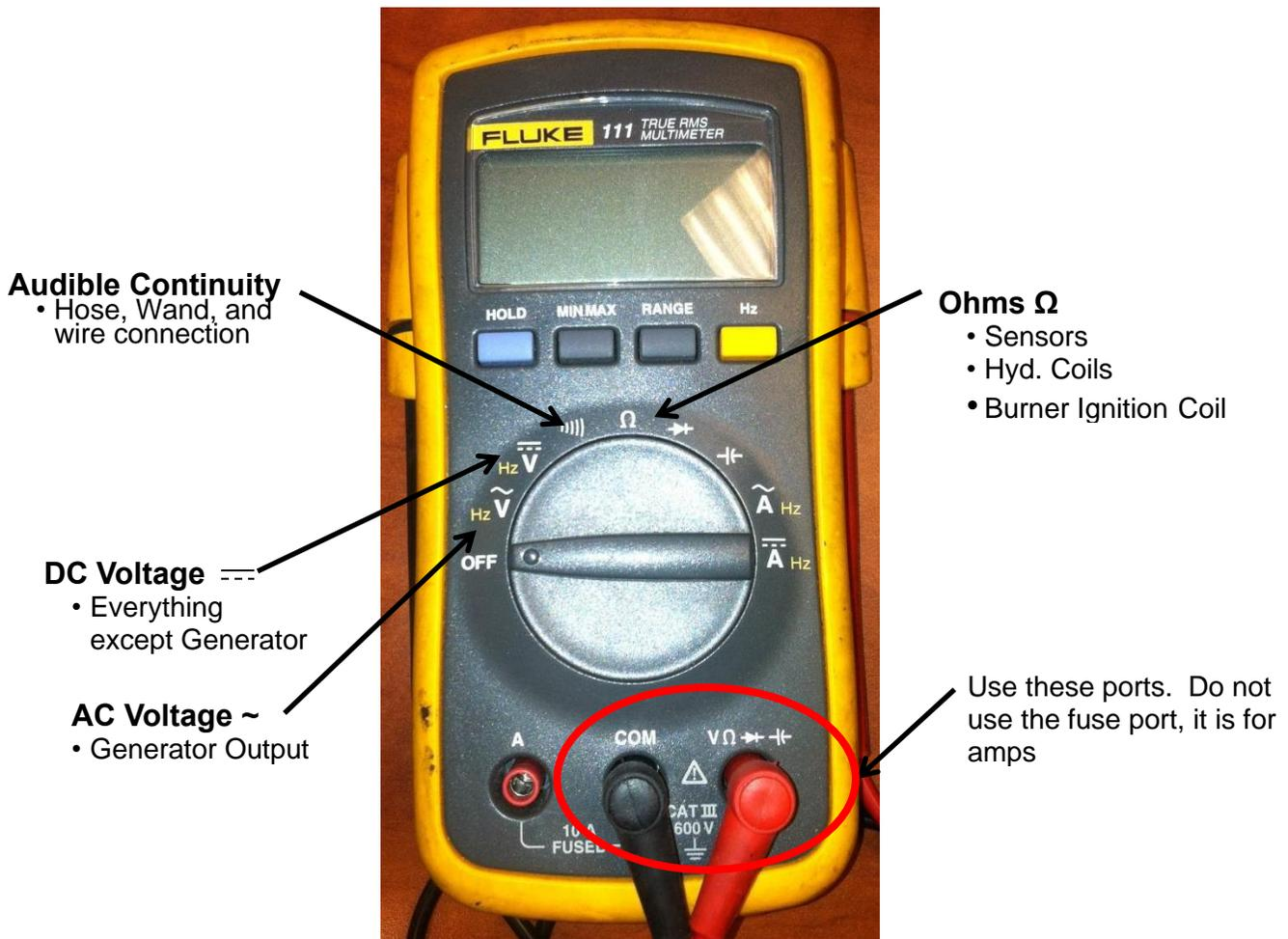
**Fig. 7-1 Standard Multimeter**
