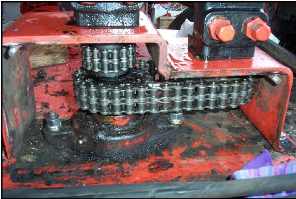
Fig. 6-15 Agitator Chain Tightening Steps
