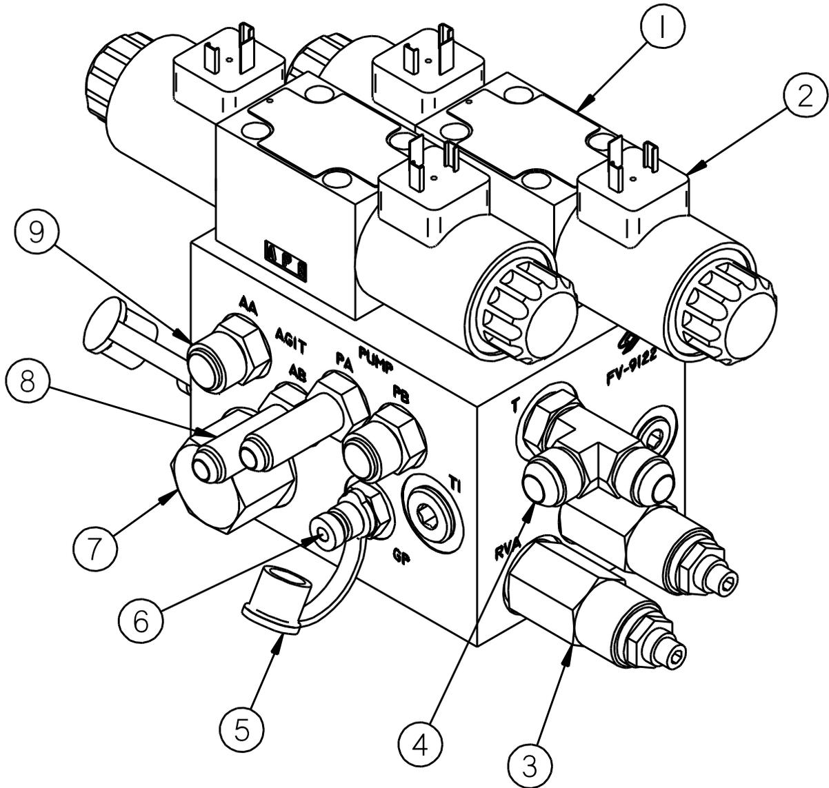
**Fig. 9-10 Hydraulic Control Valve Assembly: PN 45420 All Models**
